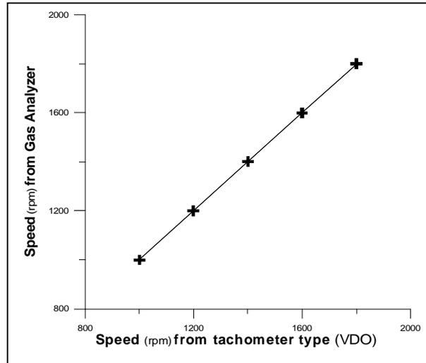
Figure (7). the tachometer calibration.
