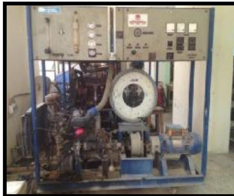
Figure (2). S.I. engine experimental rig
