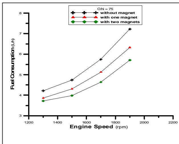
Figure (11). Fuel consumption (L/h) as a function of engine speed for fuel has octane number of 75, with and without magnetic field.
