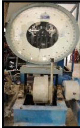
Figure (3).The hydraulic dynamometer.
