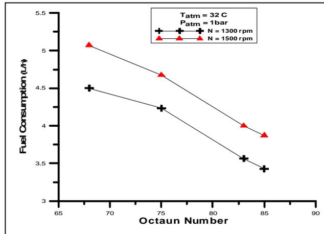
Figure (10). Fuel consumption (L/h) as a function of octane number for engine speeds (1300) and (1500) rpm without magnet.
