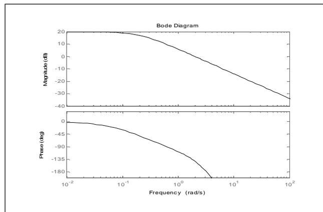
**Figure (3) Bode plot for the model p1.**
