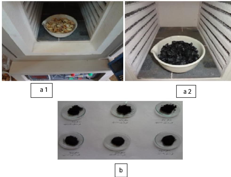
Figure.(1): Iraqi pistachio shells used in this study, (a-1) The raw pistachio shells before burn (a-2) The raw pistachio shells after burn, (b)-Granular pistachio shells carbon
