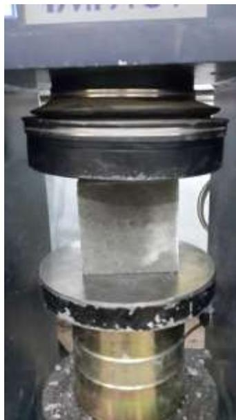
Plate (1) : Compressive strength apparatus
