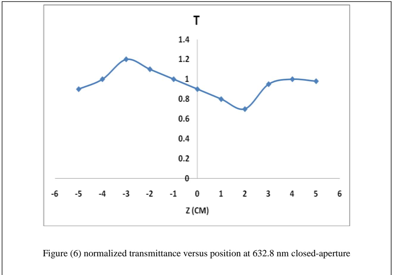
Figure (6) normalized transmittance versus position at 632.8 nm closed-aperture
