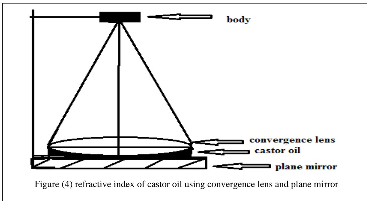
Figure (4) refractive index of castor oil using convergence lens and plane mirror
