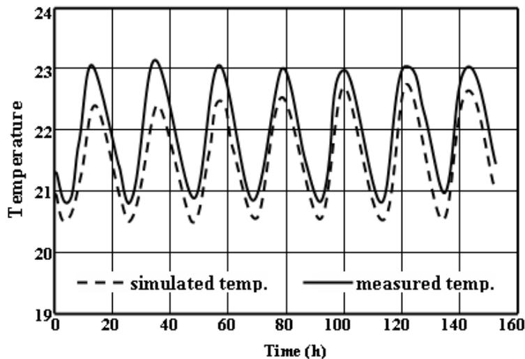
Figure (8) Surface temperature of cooling panel in test room, 16-22 August 2012
