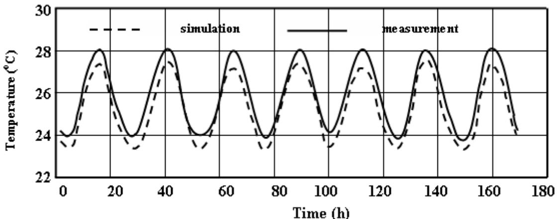
**Figure (5) Measured and simulated air temperature in test room, 16-22 august 2011**
