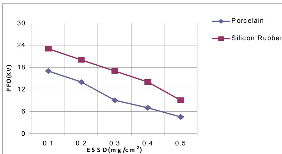
**Fig( 5 ) Flashover Voltage To ESSD For Porcelain And Silicone Rubber**
