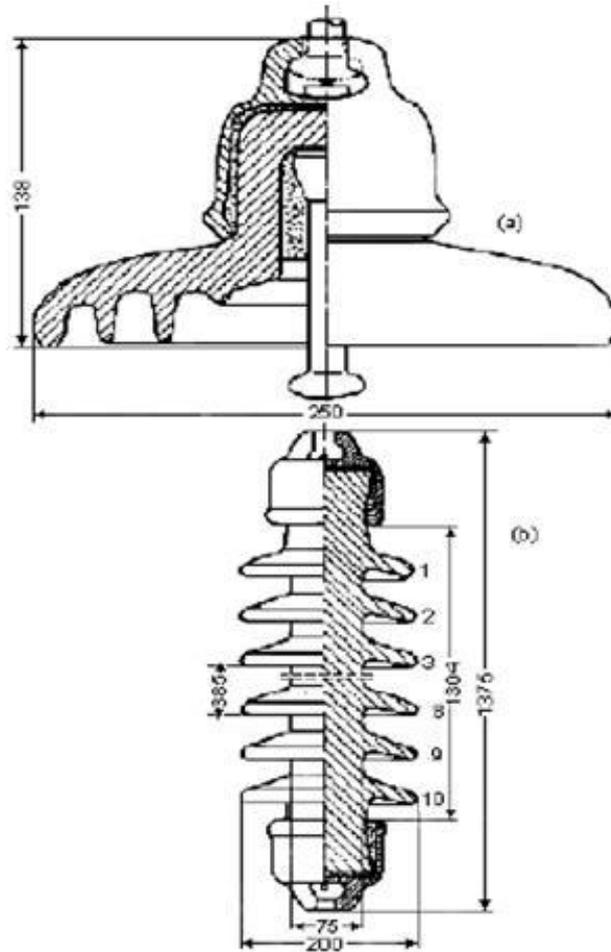
**Figure (4) Profiles Of The Insulators Tested. (A) Porcelain (Cap-Pin) Type, Leakage Path 292 Mm. (B) Silicone Rubber (Long Rod Type), Leakage Path 465 Mm And Number Of Sheds 10.**
