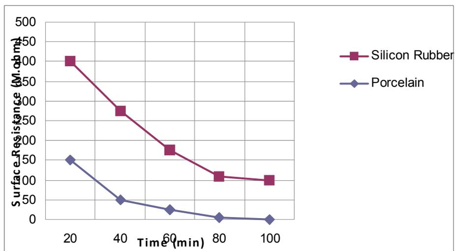
**Fig( 6 ) Surface Resistance To Time For The Insulator**
