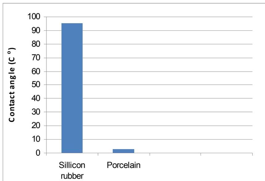
**Fig (7) The Contact Angle For The Insulator (Silicone Rubber And Porcelain)**
