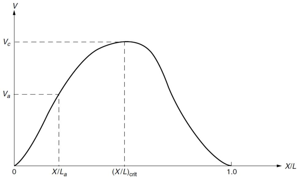
**Figure (2) Voltage Versus X/L For An Arc In Series With A Pollution Layer Of A Fixed Resistance Per Unit Length**
