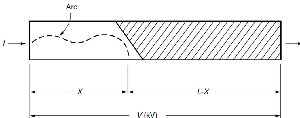
**Figure (1) Model Of A Single Arc Developing On A Polluted Surface (Uniform Pollution Layer R, KΩ/Mm)**
