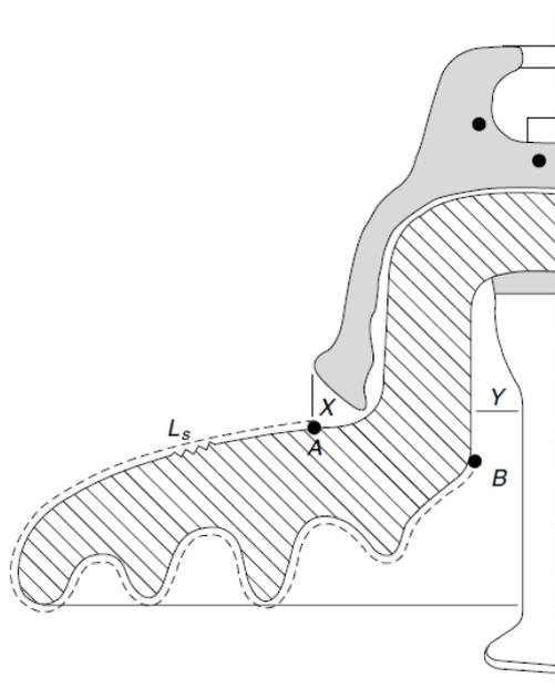
**Figure (3) Evaluation Of Insulator Dimensions For A Typical Shape.  $L_s$  = Leakage Path Length.**
