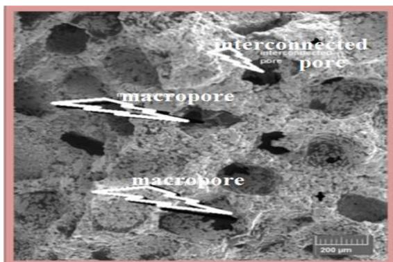
Figure 3: SEM of porous titanium sample showing the macropore
