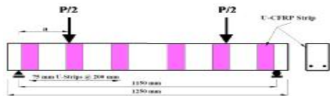
Figure (6) Shear Strengthening without End Anchoring B6 and B8
