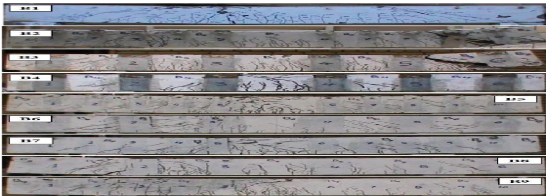
Figure. (10) Crack Patterns for tested Beams (21)
