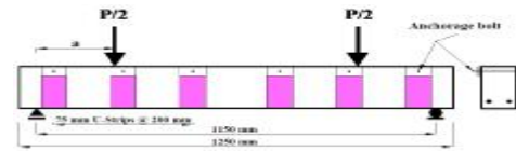
Figure (4) Shear Strengthening with End Anchoring B3 and B4 (21)
