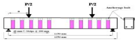
Figure (3) Shear Strengthening with End Anchoring B2 and B5 (21)
