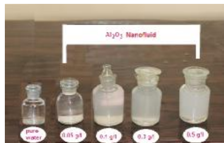
Figure (6) Photographs of the water- \text{Al}_2\text{O}_3 nanofluids preparation
