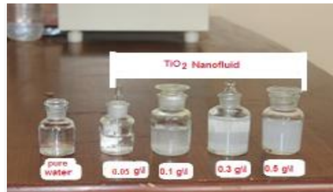
Figure (7) Photographs of the water-TiO 2 nanofluid preparation
