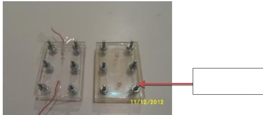
Figure (1) Photographic picture for microfluidic devices with native and coated with SiO 2 PDMS.
