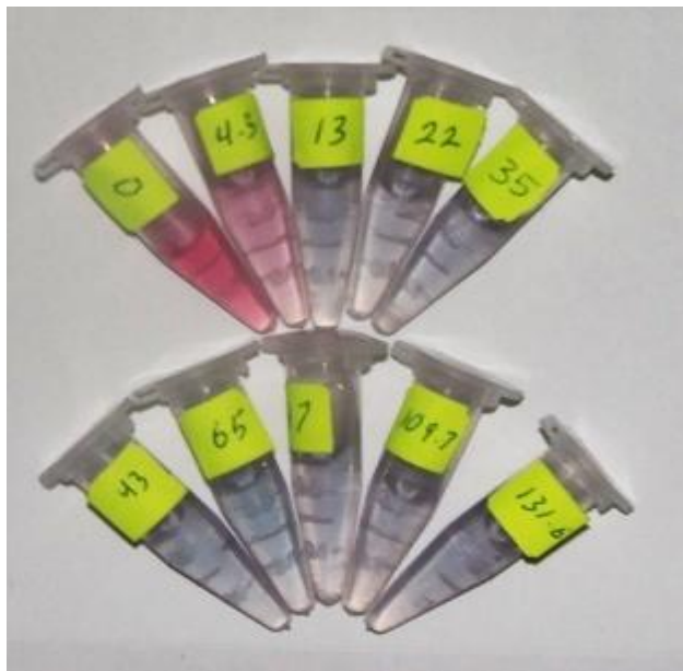
Figure (3) Photographic picture for AuNP colloid colors Changes with Cd 2+ addition.
