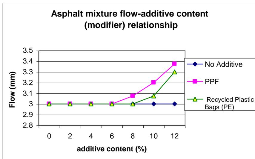
**Figure (3) Asphalt Mixture Flow – Additive Content (Modifier) Relationship.**
