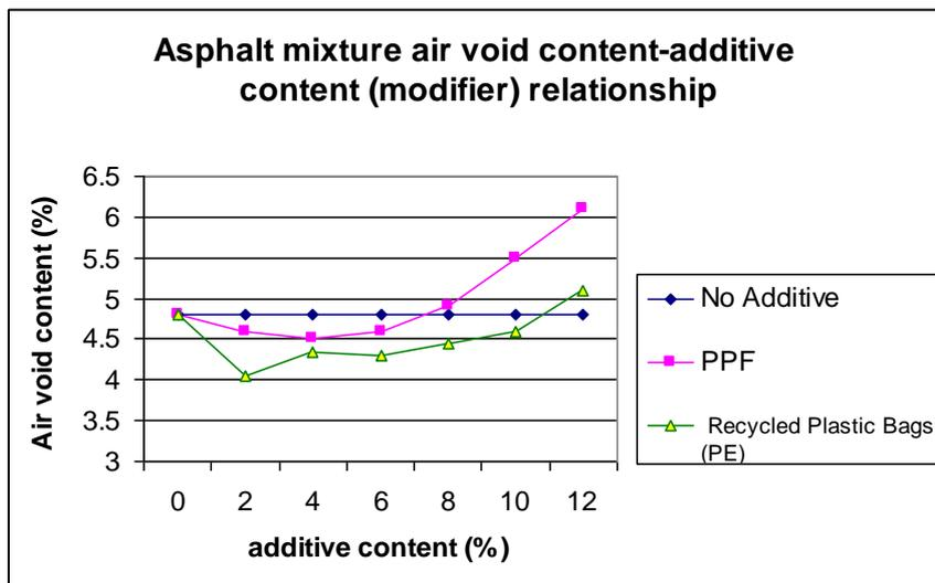
Figure (4) Asphalt Mixture Air Void Content – Additive Content (Modifier) Relationship.
