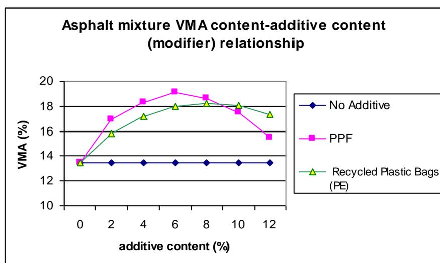
Figure (5) Asphalt Mixture VMA Percentage – Additive Content (Modifier) Relationship
