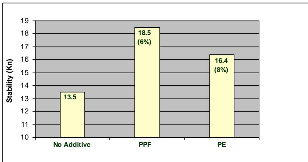
**Figure (7) Maximum Asphalt Mixture Stability by Type of Modifier.**
