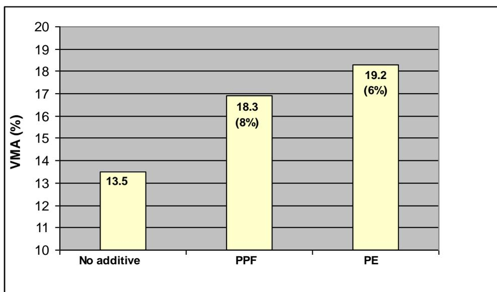
**Figure (9) Maximum Asphalt Mixture Void in Mineral Aggregate (VMA %) by Type of Modifier.**
