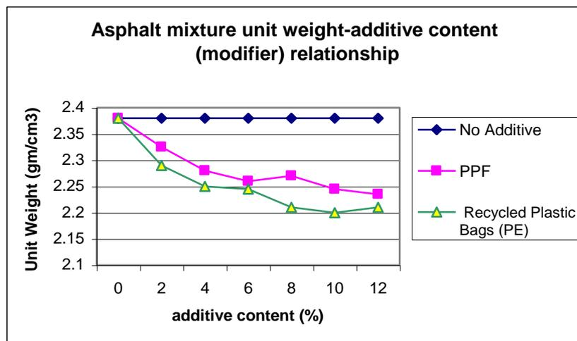
Figure (1) Asphalt Mixture Unit Weight – Additive Content (Modifier) Relationship.
