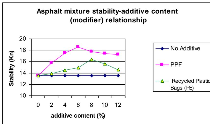
Figure (2) Asphalt Mixture Stability – Additive Content (Modifier) Relationship.
