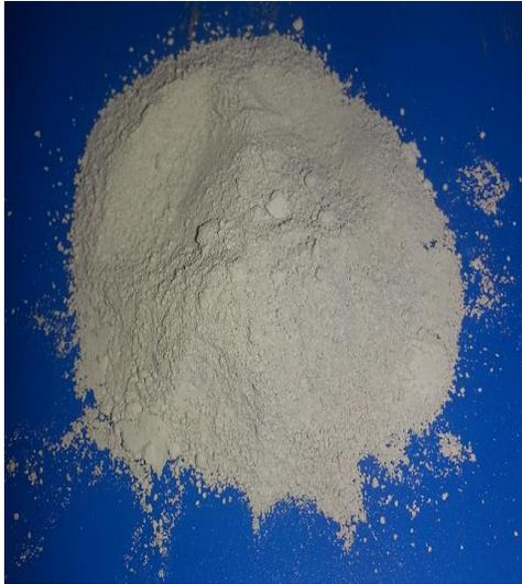
Fig. 2: Powder of cockles shells obtained by ball milling of crushed shells.
