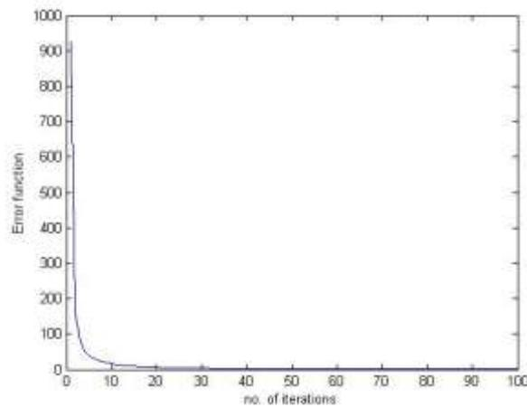
**Figure 2.** Error function versus the number of iterations when GD localization of a stationary target in 3-D space is performed using five anchor nodes. Convergence factor= $0.25$ , standard deviation (SD) of TOA measurement noise = $0.001 \mu\text{sec}$ .
