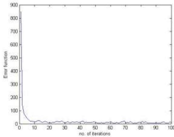
**Figure 3.** Error function versus the number of iterations when GD localization of a stationary target in 3-D space is performed using five anchor nodes. Convergence factor=0.25, SD of TOA measurement noise =0.002  $\mu$ sec and  $\mu_{\text{NLOS}}$ =0.003  $\mu$ sec.
