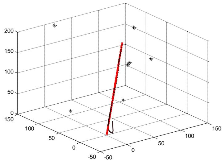
**Figure 6.** GD tracking of a moving sensor using the proposed algorithm. Initial point is [50,50,50]. Convergence factor=0.1. The basic seven anchor nodes are shown as asterisks. The true path is shown in red.
