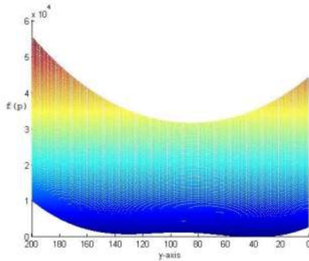
**Figure 1.** Error function  $f(p)$  as a 3-D performance surface with 2-D anchor nodes  $[10,100]$ ,  $[100,90]$ , and  $[10,70]$  and a global minimum at  $p=[60,40]$ . Azimuth= $180^\circ$  and elevation= $0^\circ$ .
