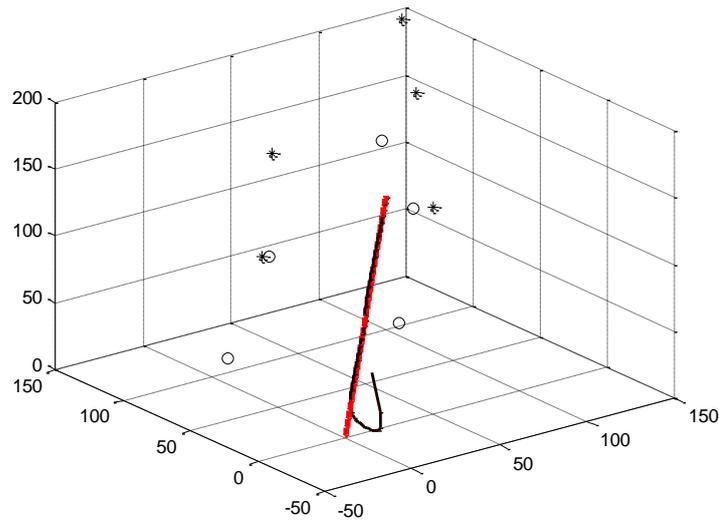
**Figure 5.** Two-segment true path and track of a moving sensor in 3-D space using iterative GD. Initial point is [50,50,50]. Convergence factor=0.1. The small circles are the 1<sup>st</sup>-segment anchors and the asterisks are the 2<sup>nd</sup>-segment anchors. The true path is shown in red.
