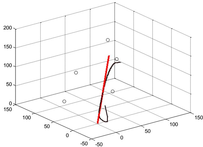
**Figure 4.** Tracking of a moving sensor in 3-D space using iterative GD with initial point [50,50,50] and a fixed set of anchor nodes (shown by the small circles). Convergence factor=0.1. The true path is shown in red.
