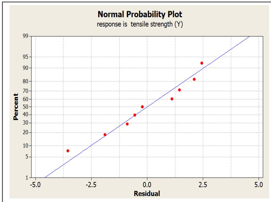
**Figure (7):** Normal probability plot of residuals of tensile strength
