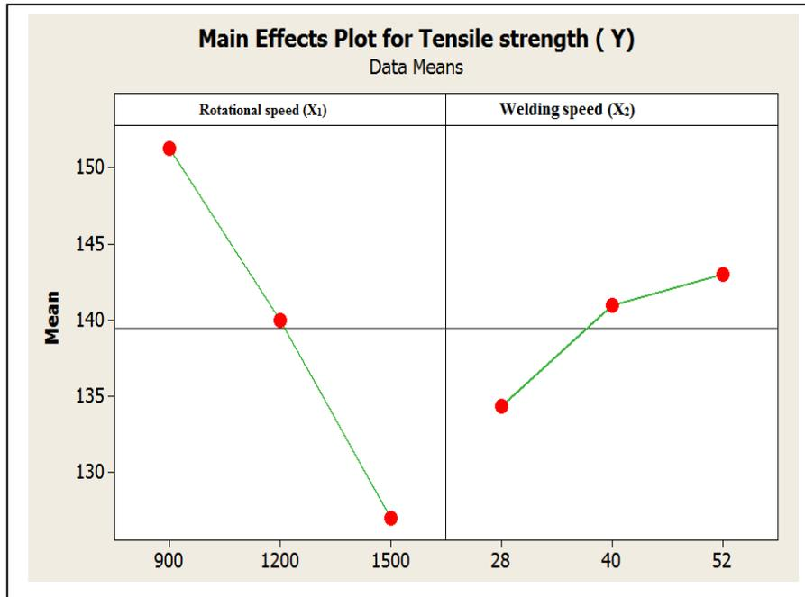
**Figure (8):** Main effect plot of residuals of tensile strength
