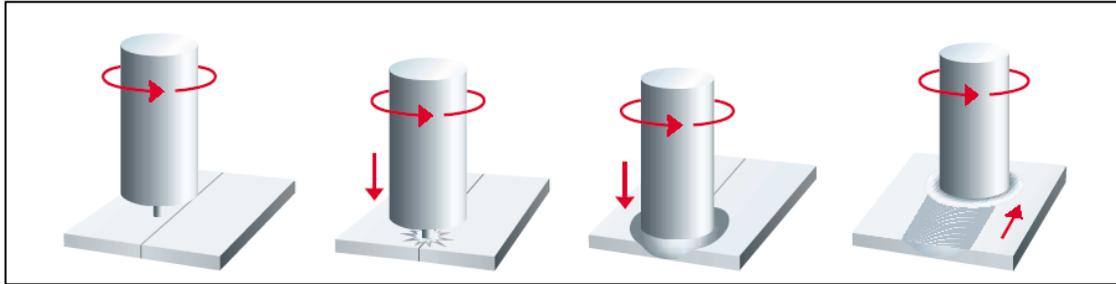
**Figure (1):** Schematic illustrations of the friction stir welding process [5].
