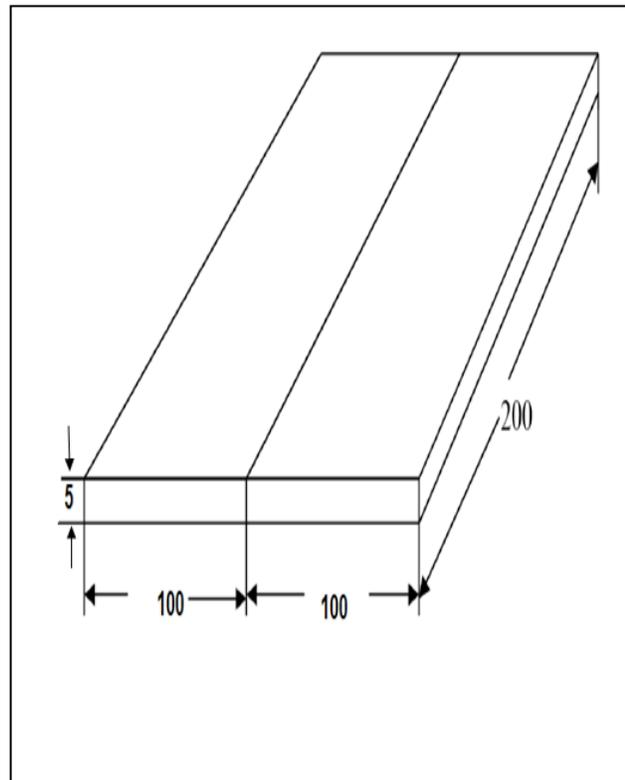
**Figure (2B):** Plate prepared for FSW.
