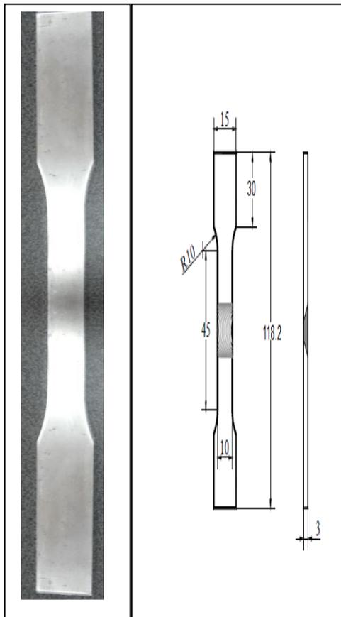
**Figure (4):** Specimen of tensile test.
