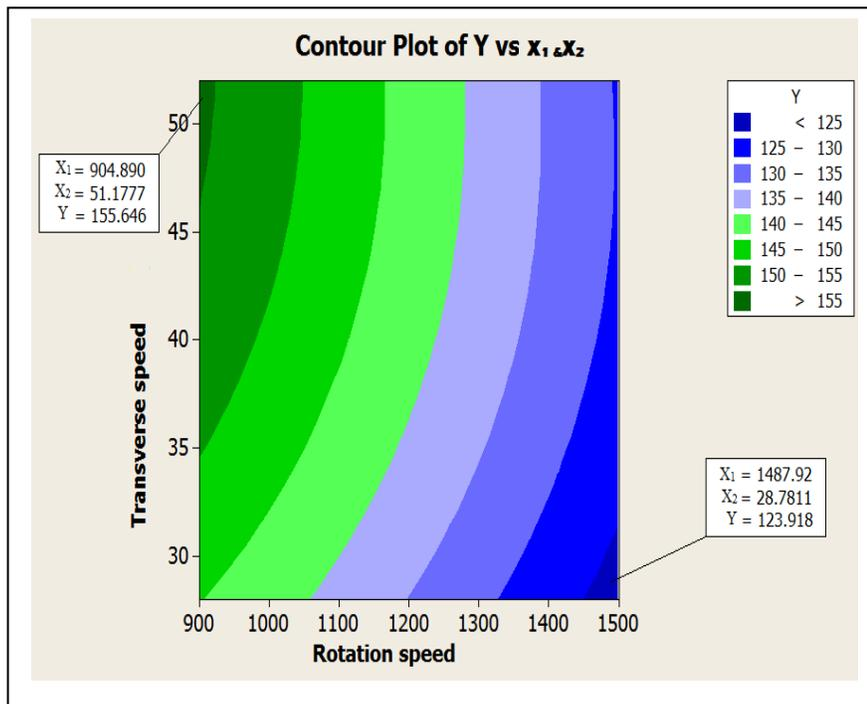
**Figure (9B):** Contour plot of tensile strength
