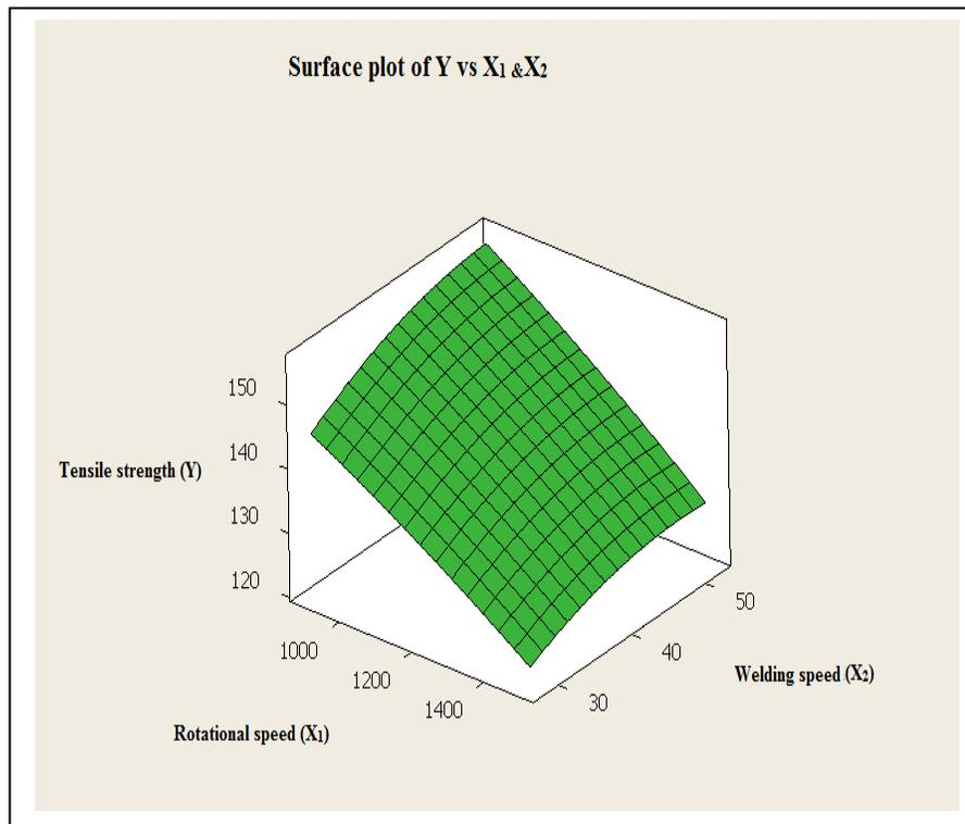
**Figure (9A):** Three-dimension plot of tensile strength
