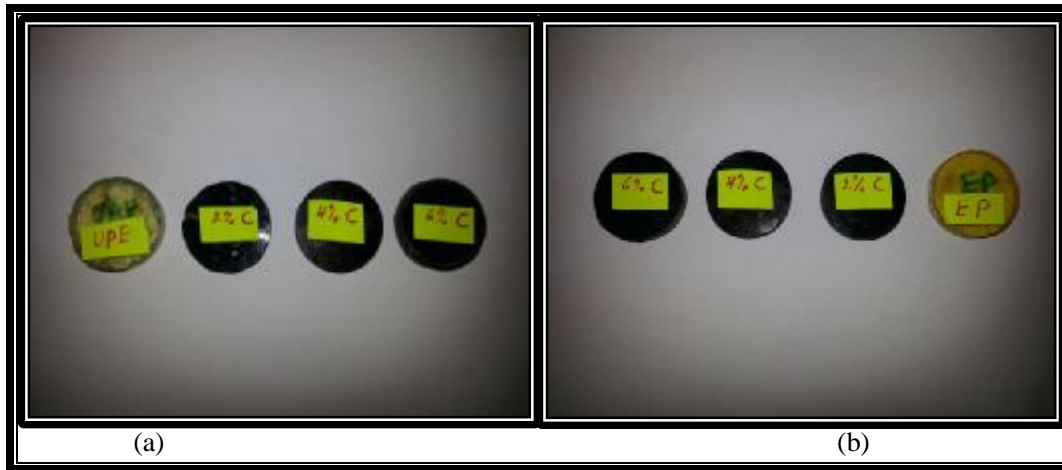
Figure (4): Photograph of thermal conductive test specimens before testing. (a) Pure polyester and TCNP/polyester nanocomposite samples. (b) Pure epoxy and TCNP/epoxy nanocomposite samples.
