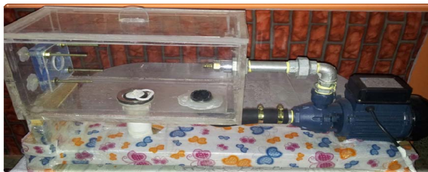
Figure (2): Erosion wear device
