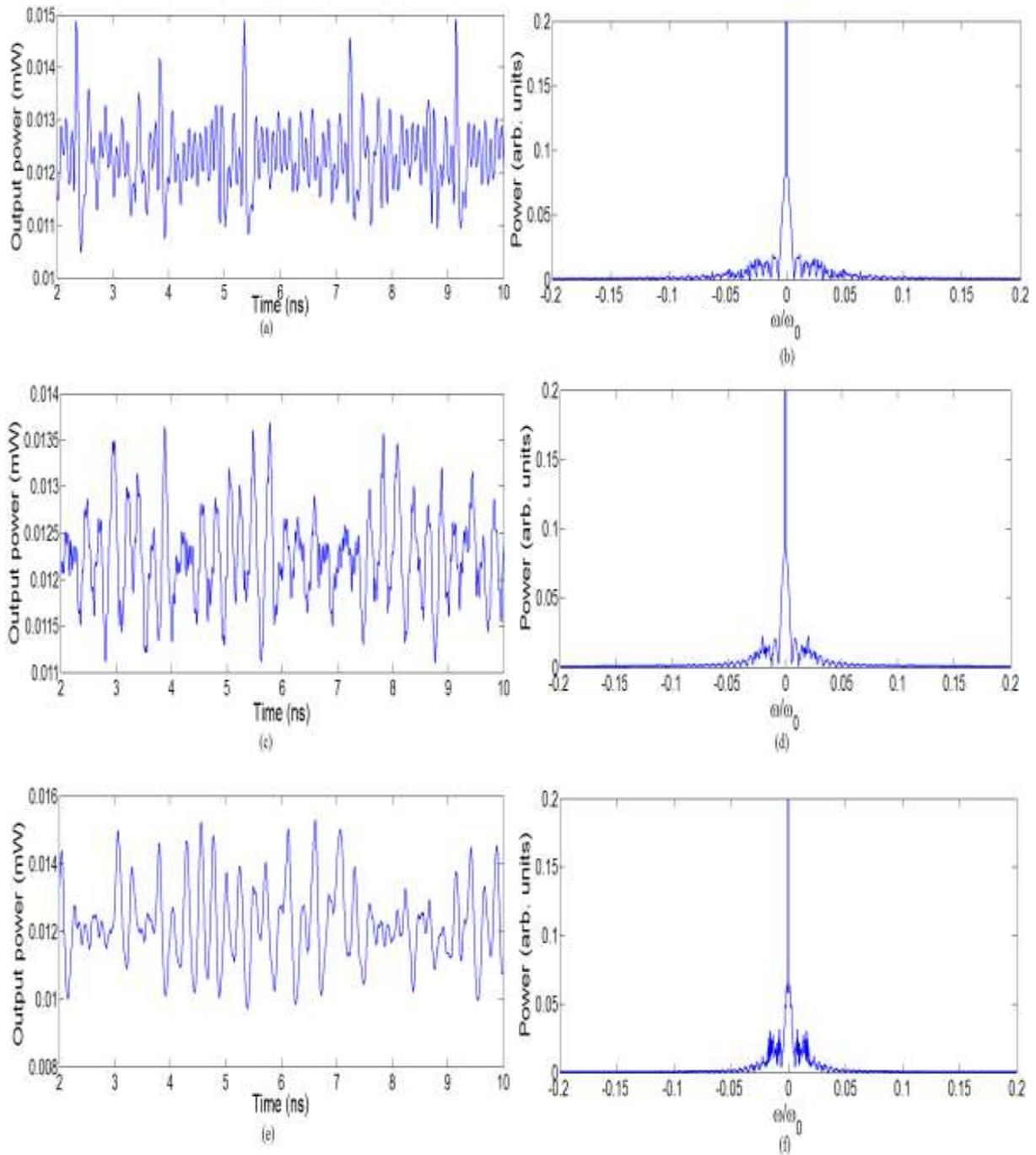
Fig (8): (Left ): Output power against time for  $m=10^{-6}$  A,  $I_0=10^{-5}$  A for the modulation frequency (10GHz , 20 GHz ,100 GHz) . (Right): The corresponding power spectrum of PC- VCSEL.
