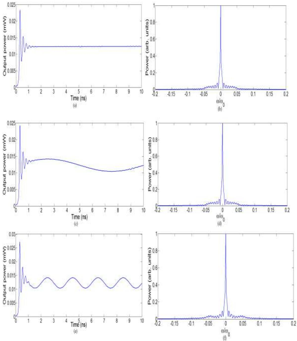
Fig (3):(Left ): Output power against time for  $m=10^{-6}$  A,  $I_0=10^{-5}$  A for the modulation frequency (0 MHz , 100 MHz ,500 MHz)(Right): The corresponding power spectrum of PC- VCSEL.
