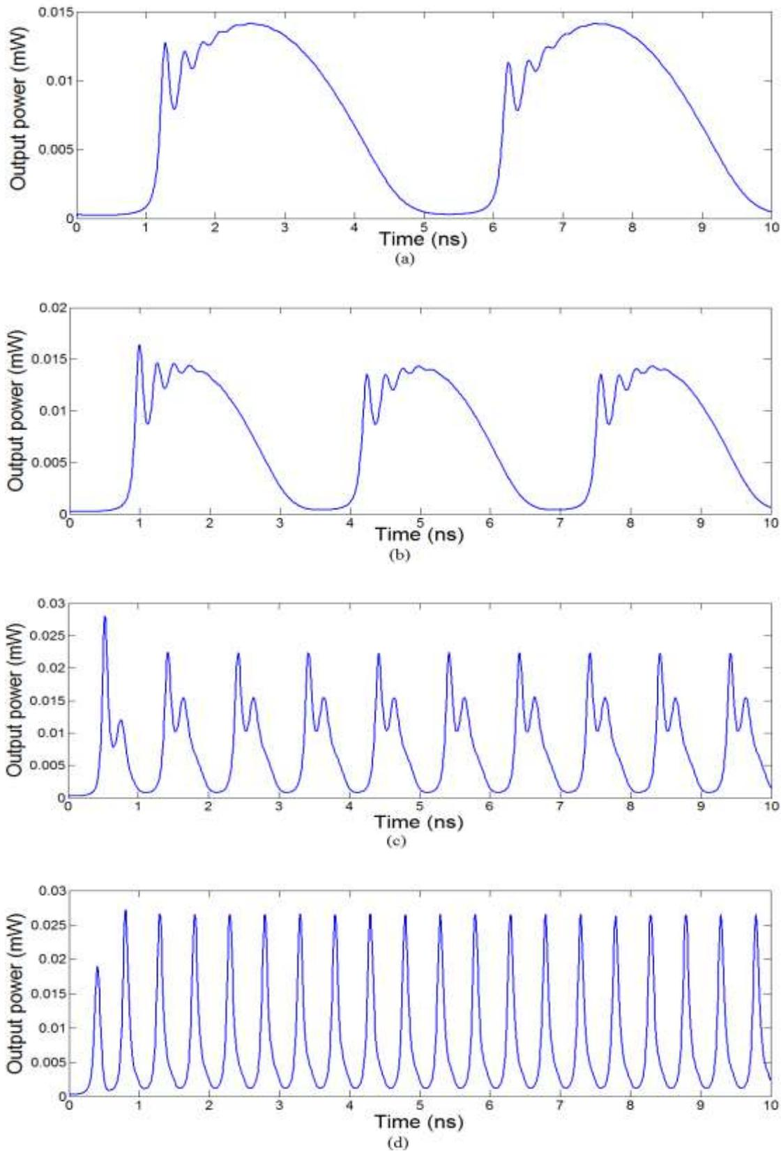
Fig(10) : Modulated output with time ,  $m = 10^{-5}$  A ,  $I_0=10^{-6}$  A , (a)  $f=100$  MHz (b)150 MHz (c) 500 MHz (d) 1 GHz
