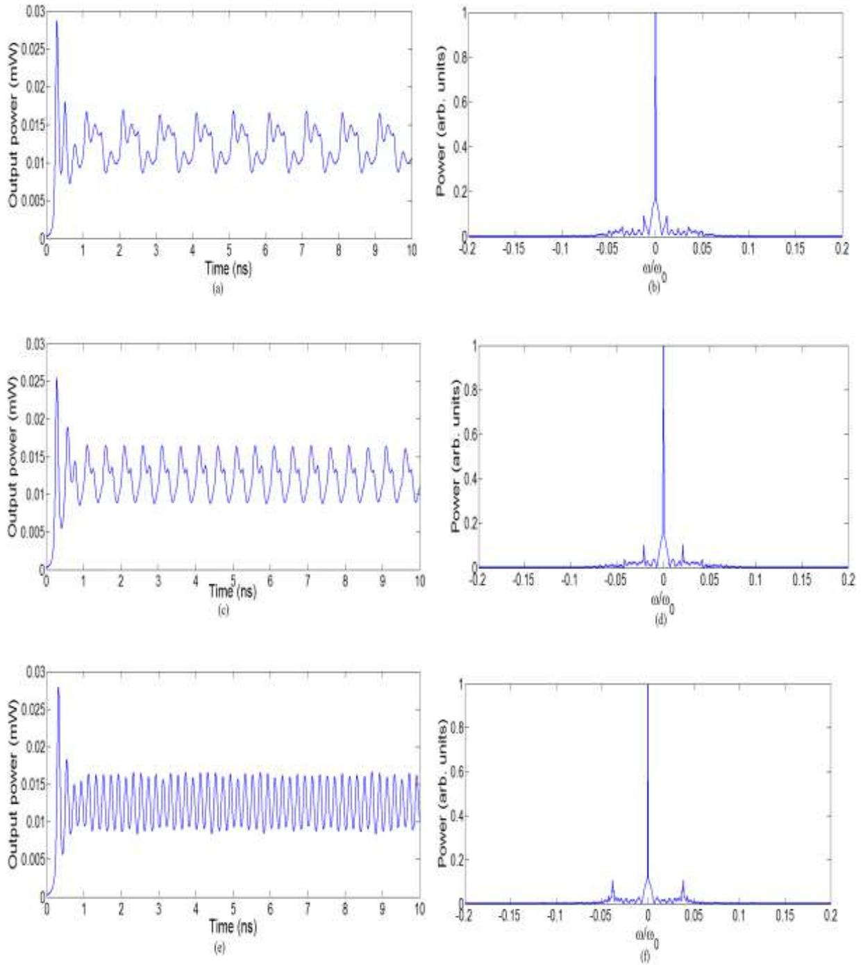
Fig (7): (Left ): Output power against time for  $m=10^{-6}$  A,  $I_0=10^{-5}$  A for the modulation frequency (1 GHz , 2GHz ,5 GHz) . (Right): The corresponding power spectrum of PC- VCSEL.
