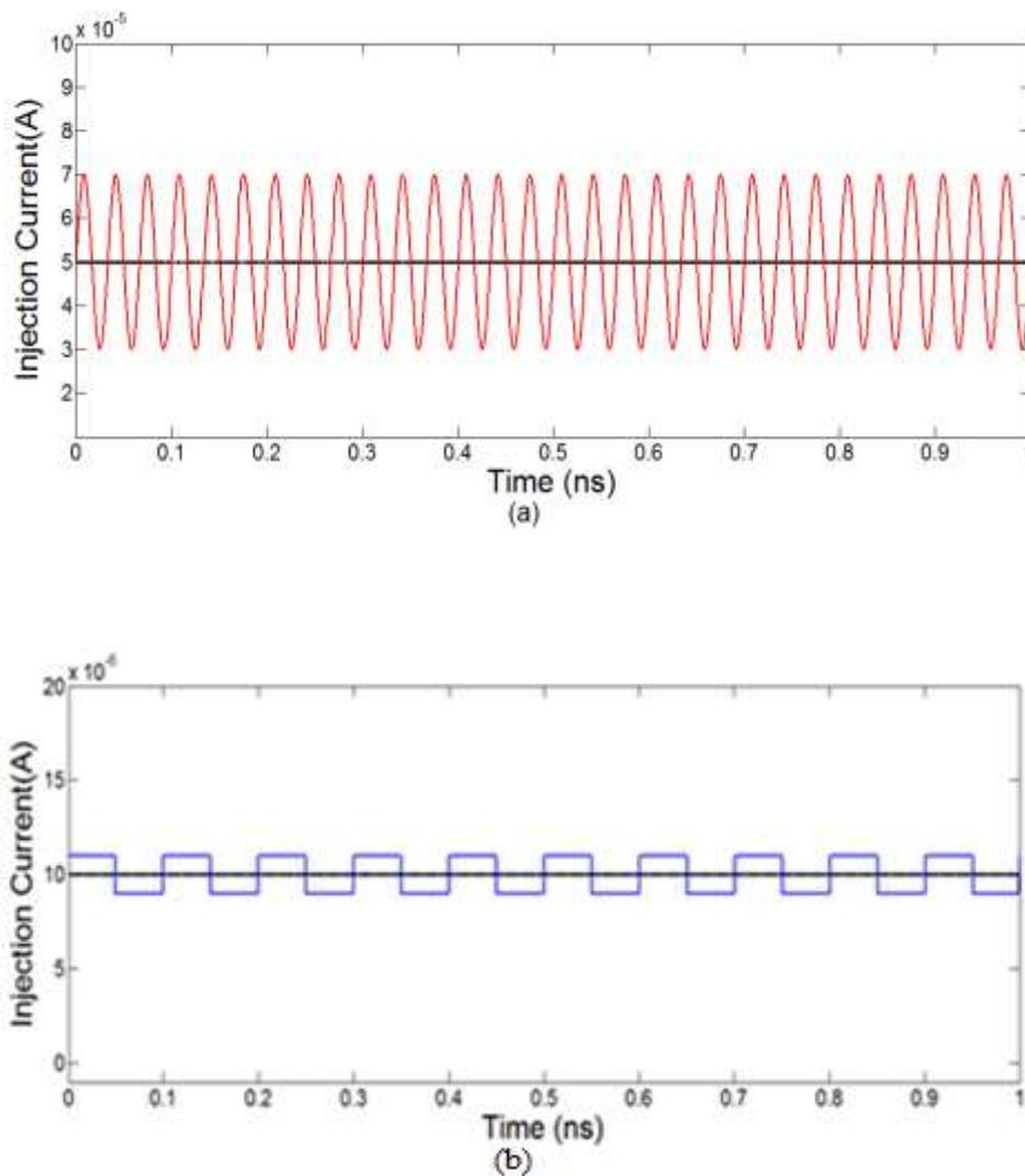
Fig (2) :Injection current against time for the modulation frequency 1 GHz (a) sinusoidal wave (b) square wave
