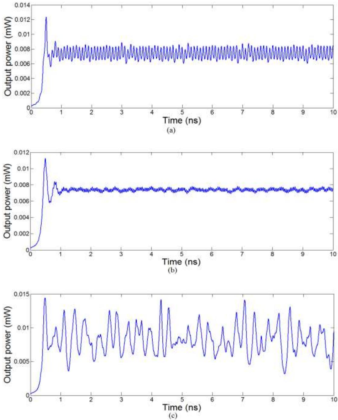
Fig(11) : Modulated output with time ,  $m = 10^{-5}$  A ,  $I_0=10^{-6}$  A , (a)  $f=5$  GHz (b)10 GHz (c) 100 GHz
