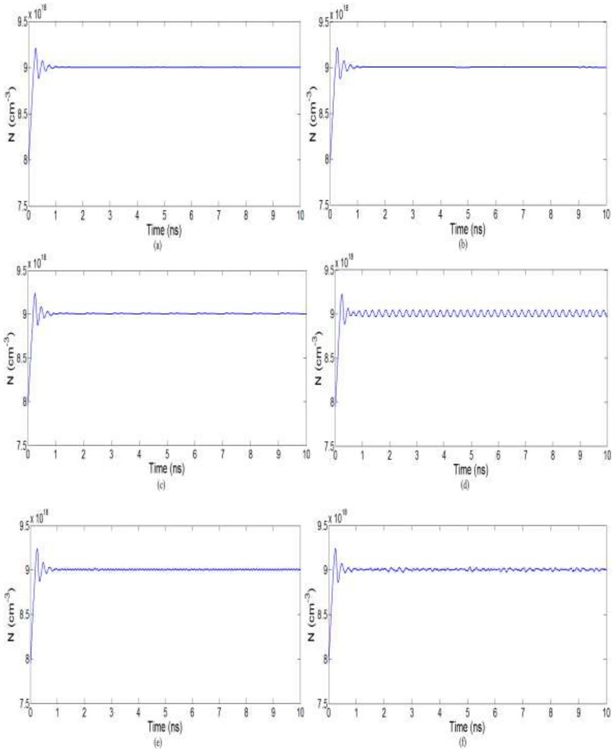
Fig (5): The variation of carriers density (N)with time at  $m=10^{-6}$  A,  $I_0=10^{-5}$  A for the modulation frequency (a) 0 MHz, (b) 100 MHz, (c)500 MHz, (d) 2GHz, (e) 5 GHz, (f) 100 GHz
