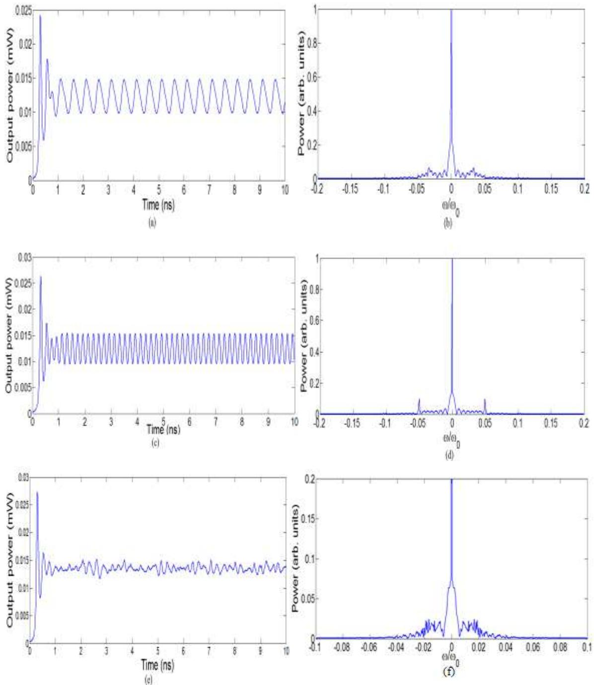
Fig (4(Left )): Output power against time for  $m=10^{-6}$  A,  $I_0=10^{-5}$  A for the modulation frequency (2GHz , 5GHz ,100 GHz) .(Right): The corresponding power spectrum of PC- VCSEL.
