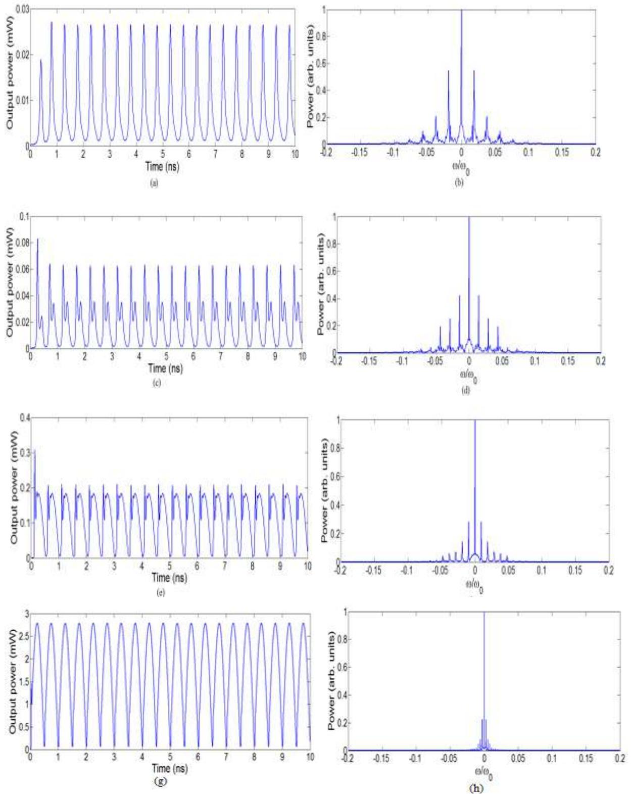
Fig (9): (Left ): Output power against time for  $f=1\text{GHz}, I_0=10^{-6}\text{ A}$
