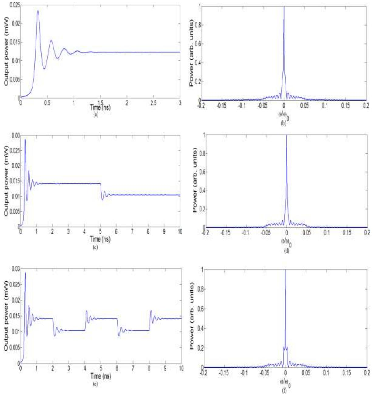
Fig (6): (Left ): Output power against time for  $m=10^{-6}$  A,  $I_0=10^{-5}$  A for the modulation frequency (0 MHz , 100 MHz ,250 MHz) . (Right): The corresponding power spectrum of PC- VCSEL.
