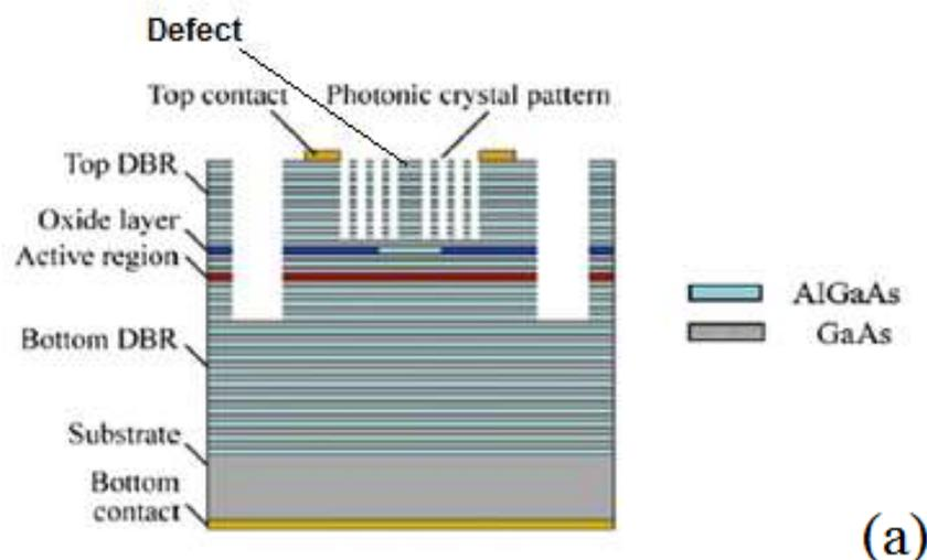
Figure 1: (a). sketch PC-VCSEL of two dimensional Photonic crystal (b) Single-defect photonic crystal cavity laser
