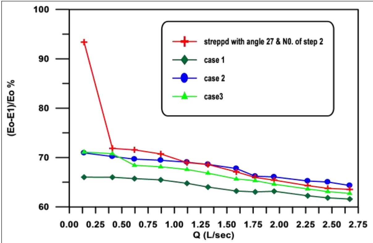
**Fig.(13): Relations between relative energy dissipation and discharges for the three cases and model No. 4.**
