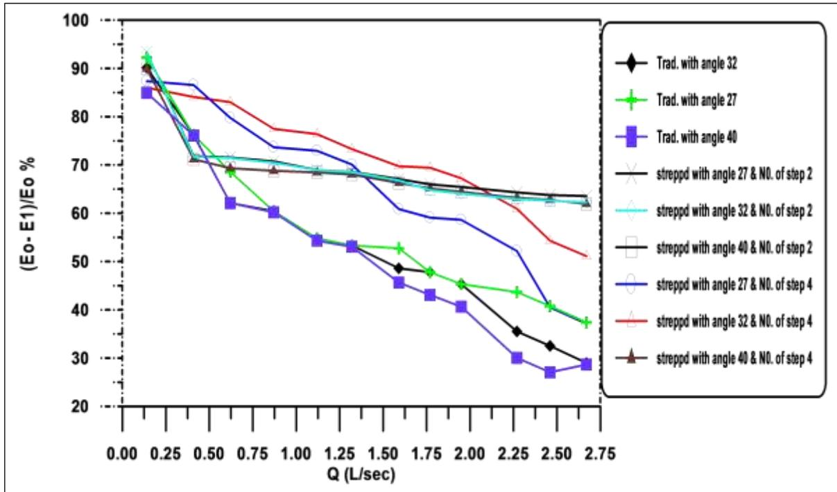
**Fig.(6): Relations between discharge and relative energy dissipation.**
