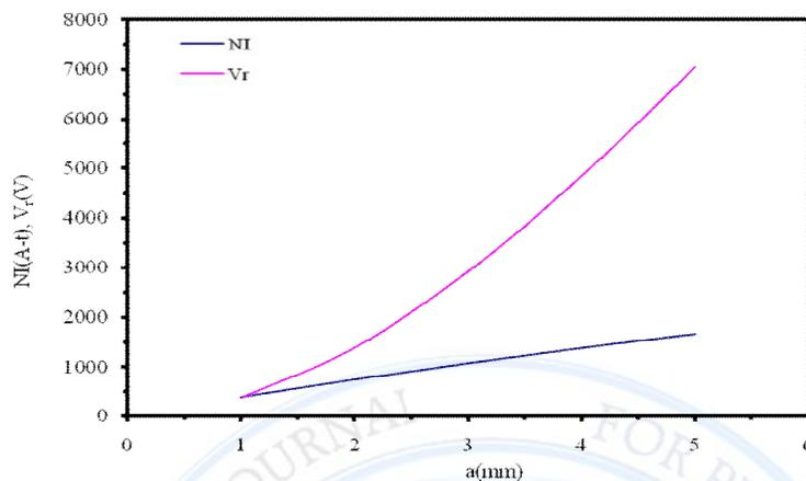
**Figure 2: Magnetic field parameter NI and  $V_r$  as a function of a.**
