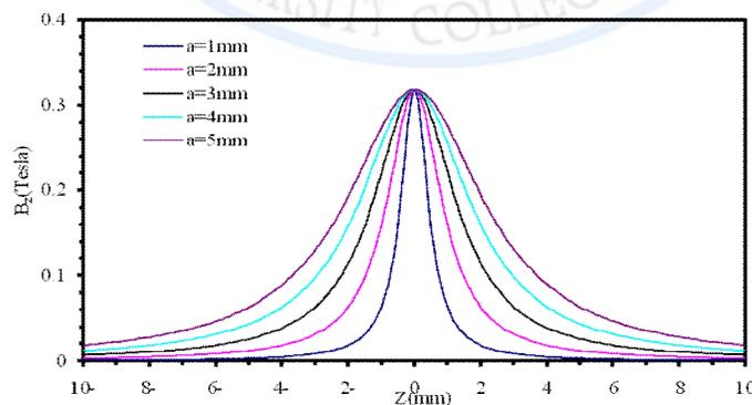
**Figure 1: The magnetic field distribution  $B_z$  at different values of  $a$ .**
