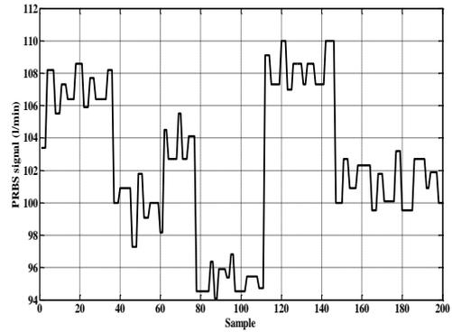
Figure (5-a): The PRBS input signal used to excite the system.
