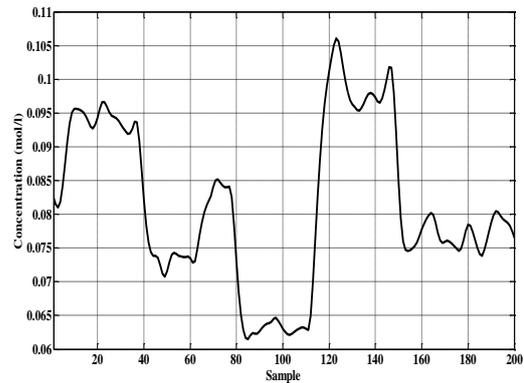
Figure (5-b): The CSTR open loop response to the PRBS input signal.
