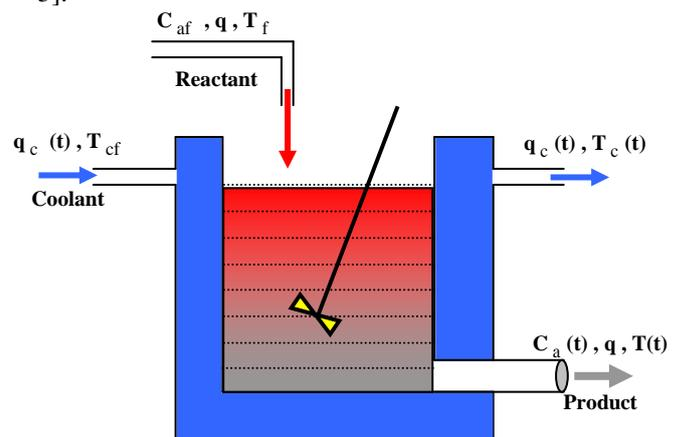
Figure 1: CSTR with cooling jacket [4,5].
