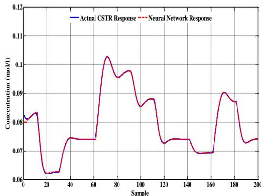
**Figure 8:** Neural network output and actual CSTR output for testing set.
