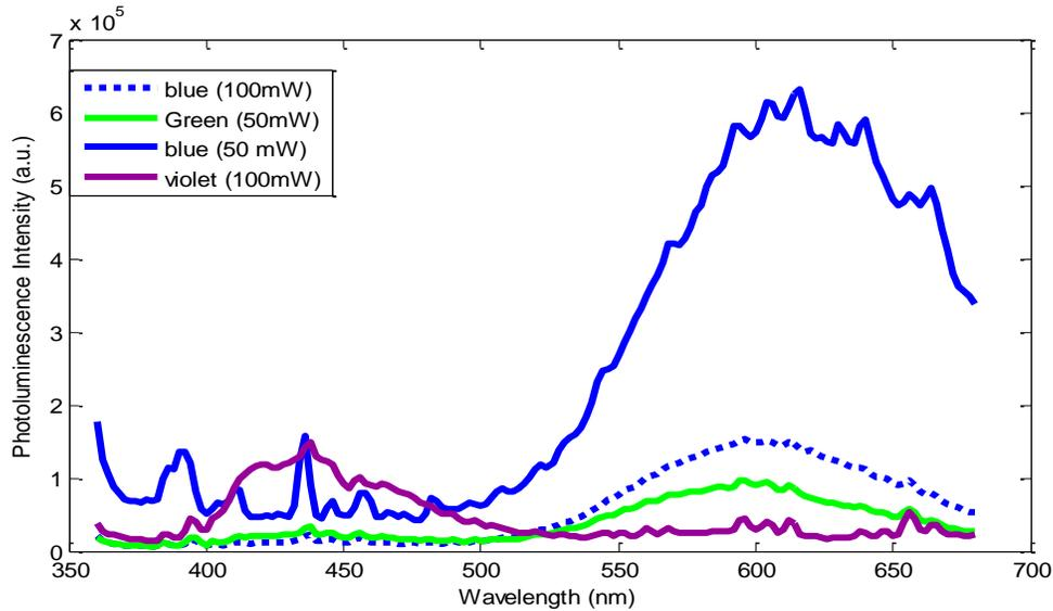
**Figure 6:** Photoluminescence spectrum of the p-n junction porous sample prepared by different lasers (Blue, Green ,Violet ) at 15min.
