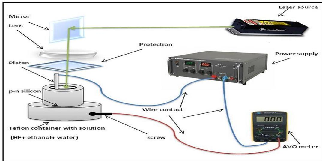
**Figure 1:** The PEC system (schematic diagram)
