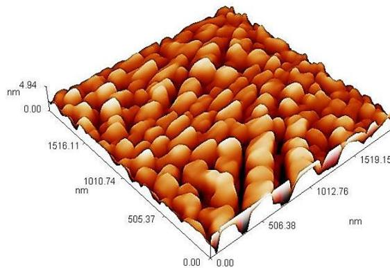
**Figure 5:** AFM image of porous silicon monolayer prepared at  $J=15 \text{ mA/cm}^2$  etched under 15 min and blue laser=50mW
