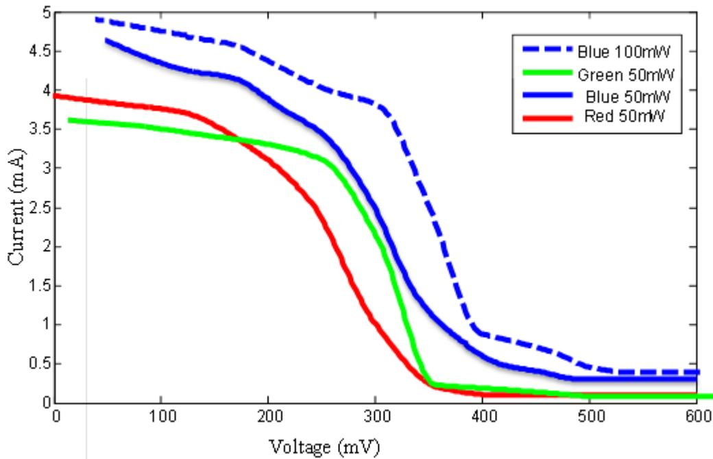
**Figure 2:** Electrical characteristics of the nanostructured solar cells produced at different wavelengths (473,532 & 671) nm at {50&100mW} powers.
