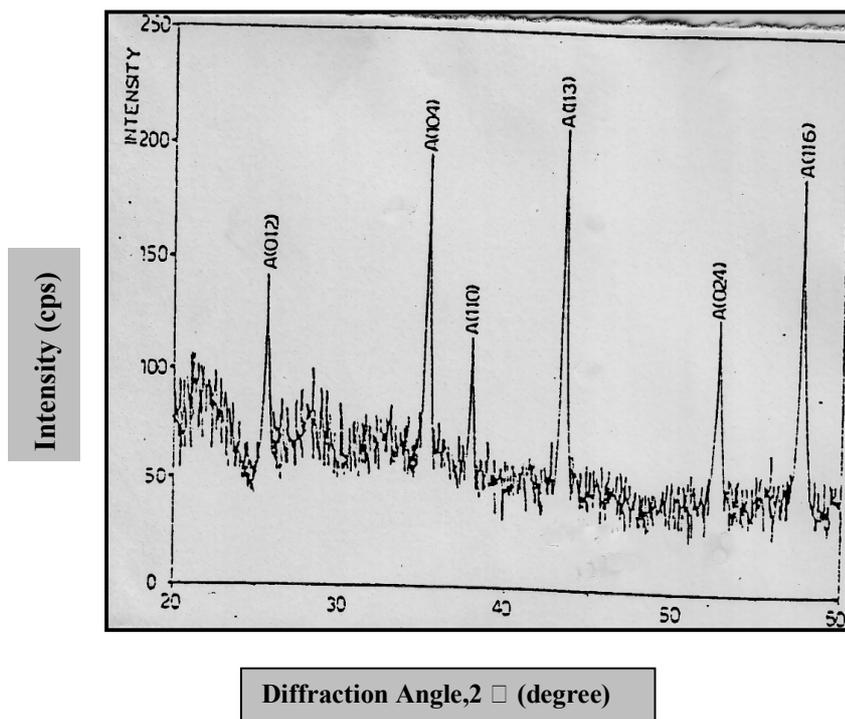
Fig. 2: Diffractograms from the surface of chopped alumina fibers ( $\text{Al}_2\text{O}_3$ )
