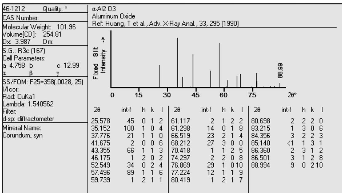
Fig. 3: Standard Diffractograms of  $\alpha$ - $\text{Al}_2\text{O}_3$
