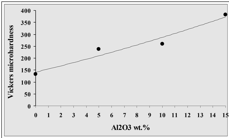
Fig. 4: Vickers micro hardness vs. chopped alumina fibers (Al<sub>2</sub>O<sub>3</sub>wt.%)
