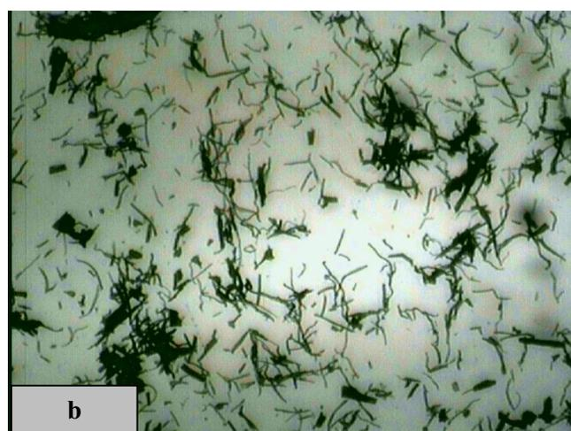
**Figures 1a and b: Light optical microscopy images of chopped alumina fibers which prepared in this work(Magnification 400X).**
