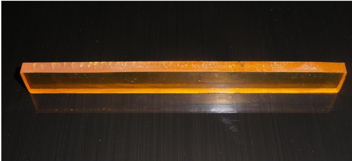
Figure 1. Pure bending test specimen.
