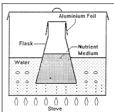
Fig. 3. A way of sterilization of flasks and nutrients medium.
