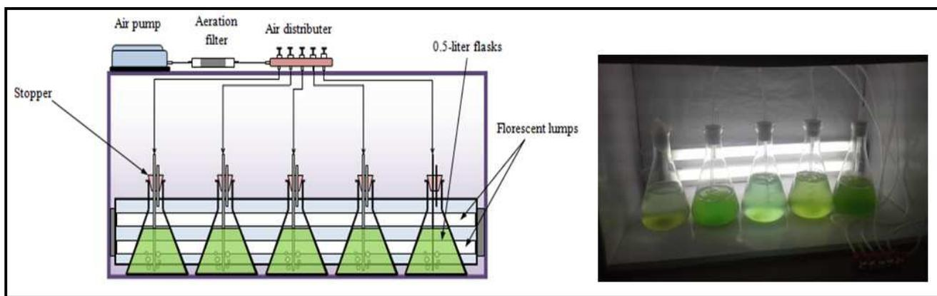
Fig.1. Experimental setup of *Chlorella vulgaris* strain incubate
