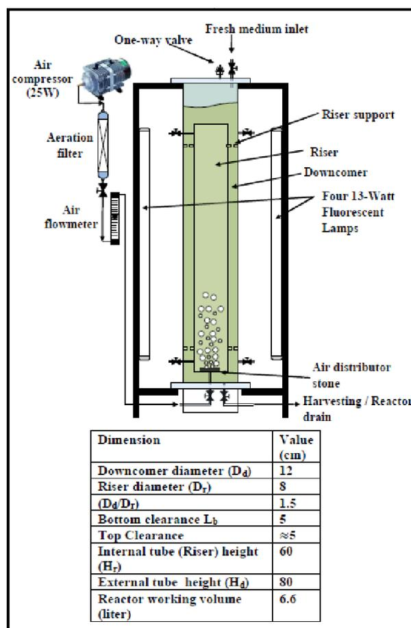
Fig. 5. Laboratory airlift photobioreactor schematic.
