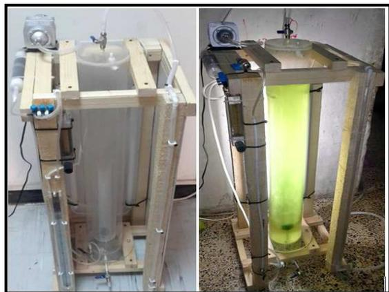
Fig. 6. photographic view of the laboratory airlift photobioreactor in use.
