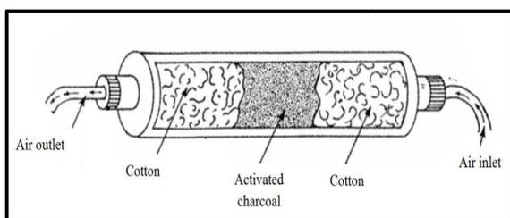
Fig. 4. Aeration filter used in avoid contamination in the air lines.
