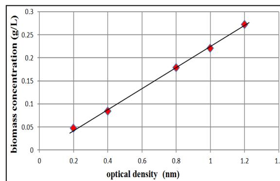
Fig. 8. Calibration curve for relationship between optical density and cell dry weight.
