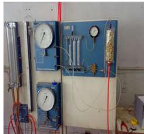
**Figure (2):** Constant head permeameter (After Todd, 1959)
