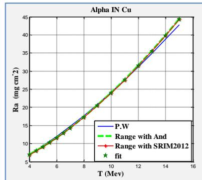
Figure (1)the range of alpha particle in Cu
