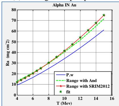
Figure (6) the range of alpha particle in Au
