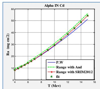
Figure (4)the range of alpha particle in Cd
