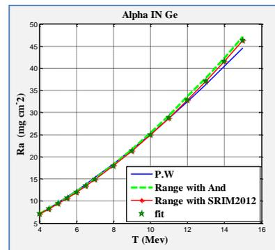
Figure (2)the range of alpha particle in Ge
