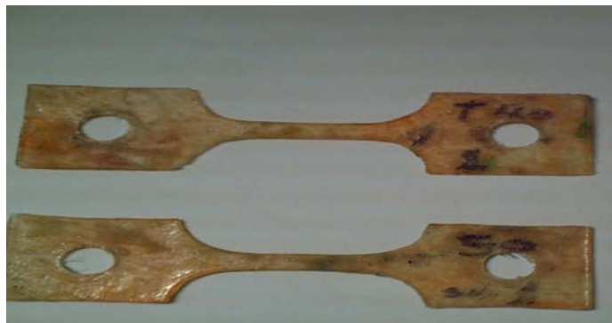
Figure.(5) Photograph of composite creep test specimen
