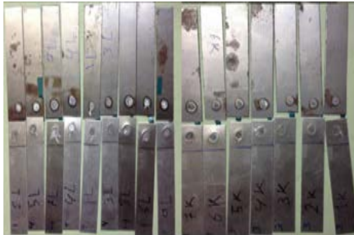
Figure (5) the tested shear force specimens.
