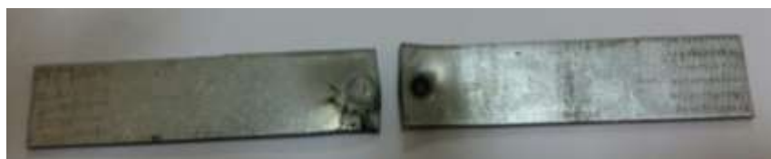
Figure (6): Fractured shear test specimen
