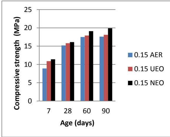
Fig. 4. Compressive strength of concrete mixes containing 0.15 dosage of different air entraining agent with time
