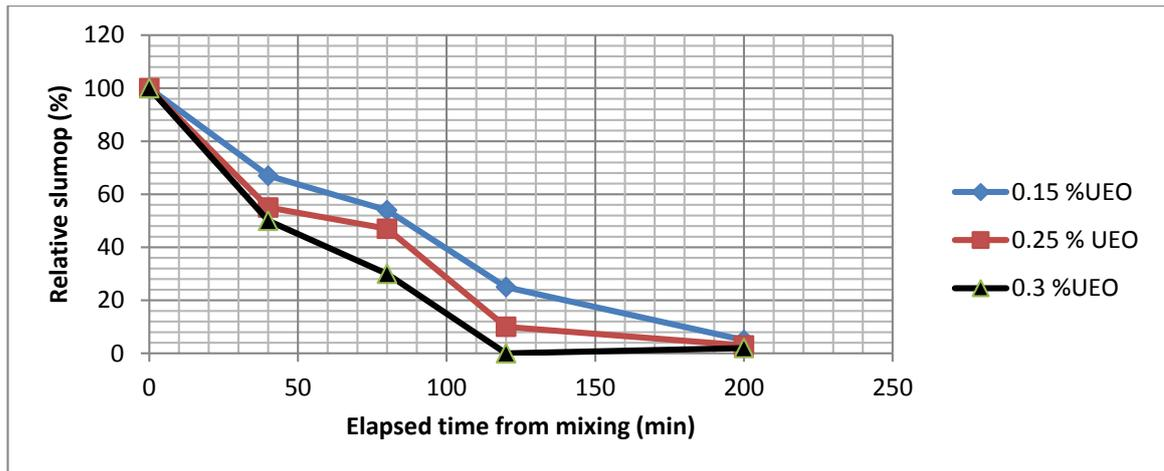
Fig. 3. Rate of slump loss of OPC concrete mixes made with different contents of UEO
