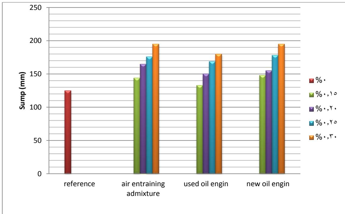
Fig. 1. Variation of slump (mm) of concrete mixes containing different admixtures
