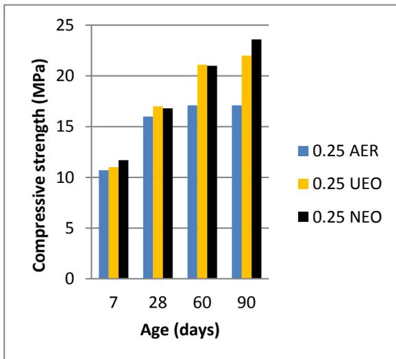
Fig. 6. Compressive strength of concrete mixes containing 0.25 dosage of different air entraining agent with time
