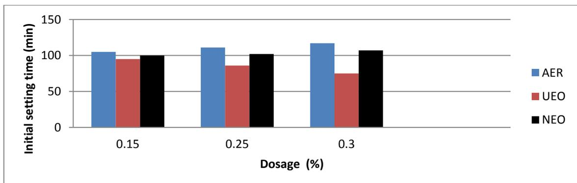
Fig. 2. Initial setting time of OPC mixes made with various admixtures
