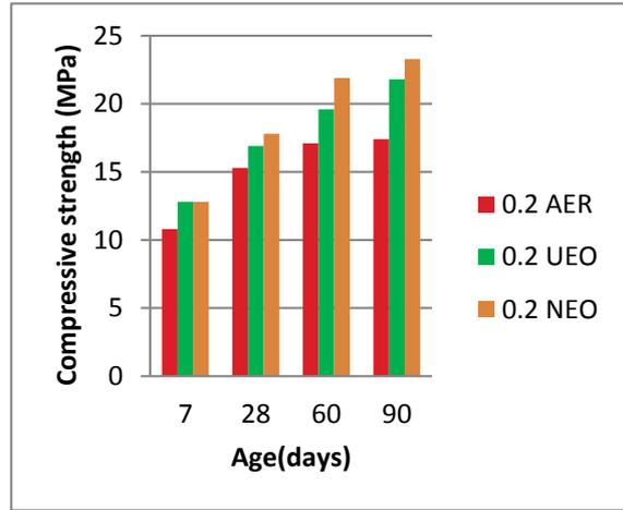
Fig. 5. Compressive strength of concrete mixes containing 0.2 dosage of different air entraining agent with time
