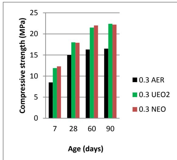
Fig. 7. Compressive strength of concrete mixes containing 0.3 dosage of different air entraining agent with time
