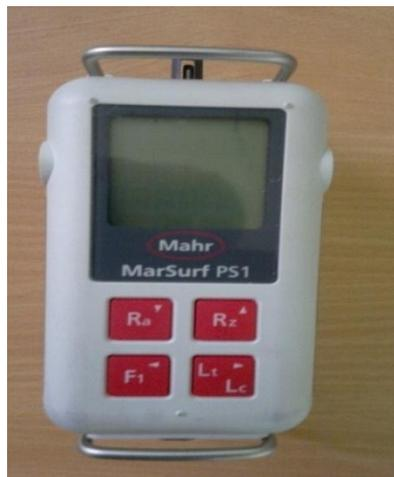
**Figure 7:** The Surface Roughness Tester
