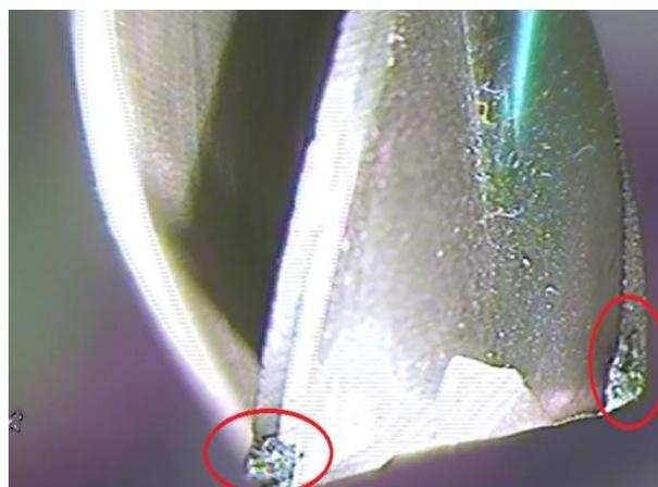
**Figure 8:** Shown the Catastrophic Failure Wear Type
