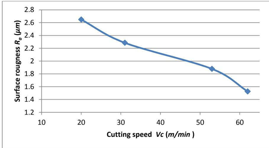
Figure 9: The Relationship between Cutting Speed and Surface Roughness
