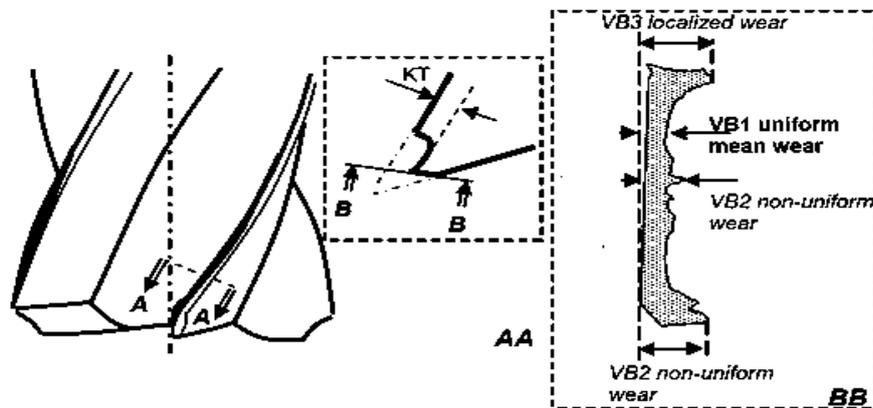
**Figure 1:** Wear of end milling tools [4]
