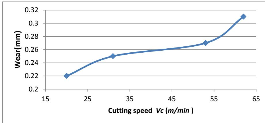
**Figure 6:** The Relationship between Wear and Cutting Speed
