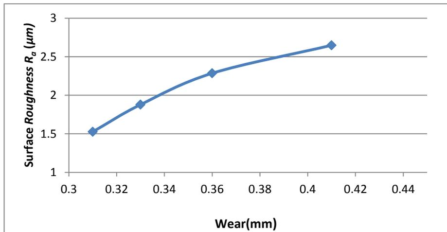
Figure 10: The Relationship between Wear and Surface Roughness
