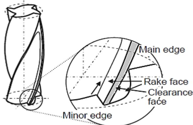
**Figure 2:** Basic geometry of end milling tools [4]
