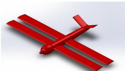
**Figure 1:** Tandem-wing UAV by using AutoCAD software
