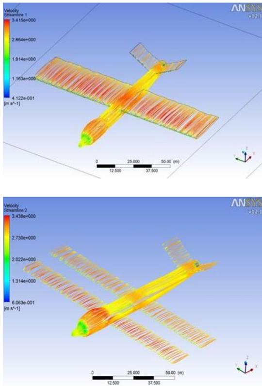
**Figure 9:** The comparison of The Velocity between the two models.
