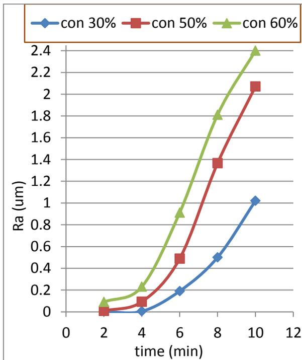
**Figure (3) Effect of machining time on Ra**
