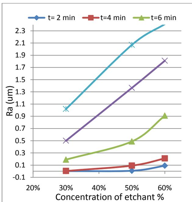
Figure (5) Effect of etchant concentration on Ra
