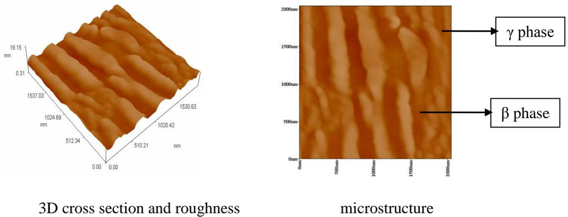
**Figure (7) Surface roughness and microstructure for the samples before CHM**
