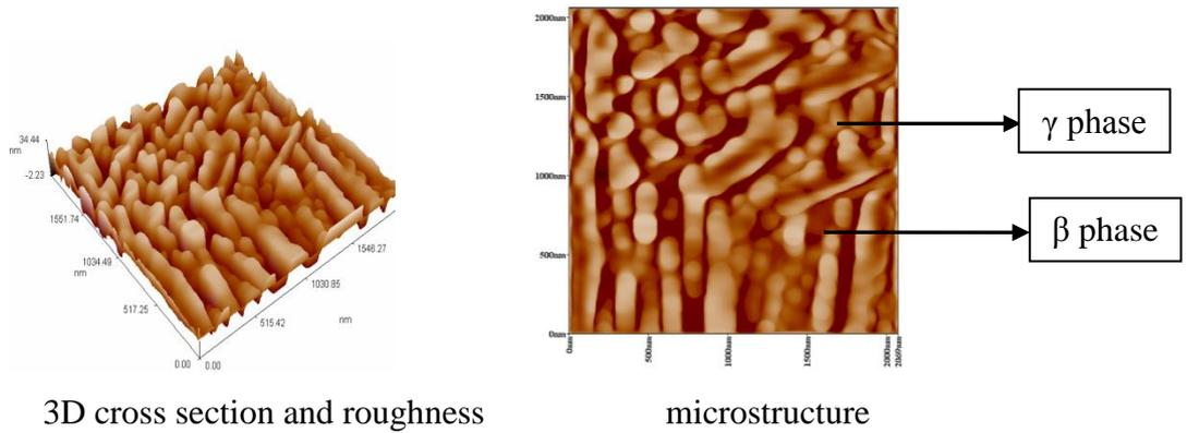
**Figure (9) Surface roughness and microstructure for the samples after CHM with concentration 50%**
