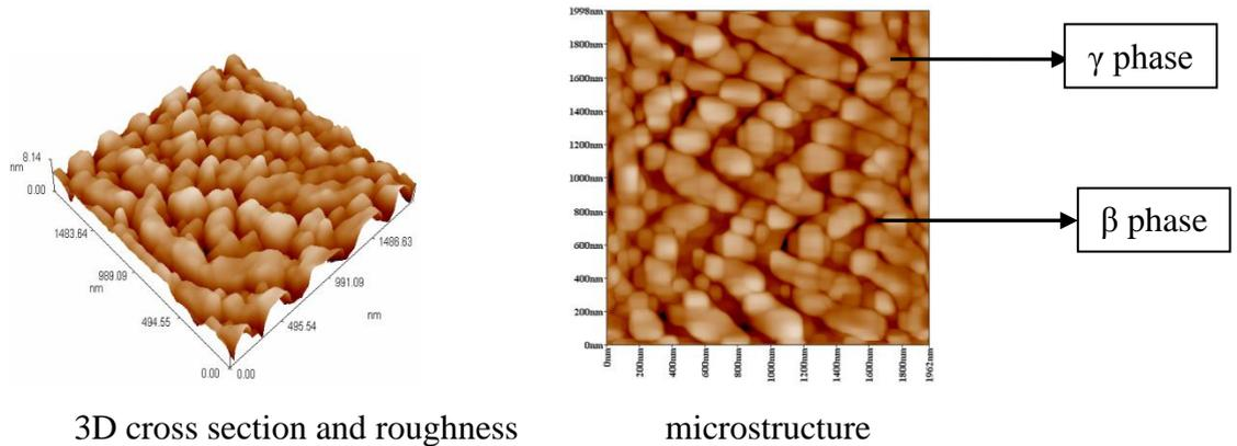
**Figure (10) Surface roughness and microstructure for the samples after CHM with concentration 60%**
