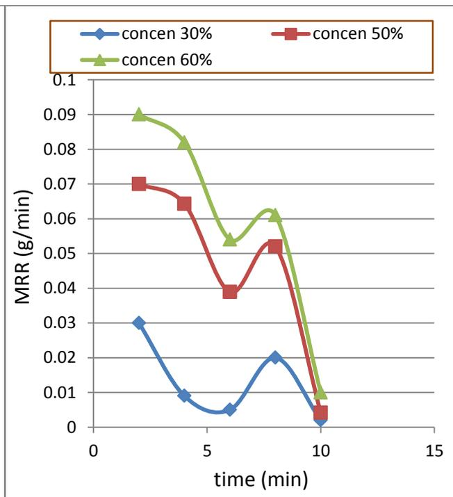
**Figure (4) Effect of machining time on MRR**
