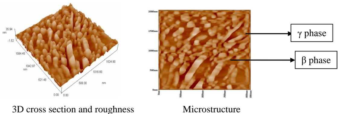
**Figure (8) Surface roughness and microstructure for the samples after CHM with concentration 30%**
