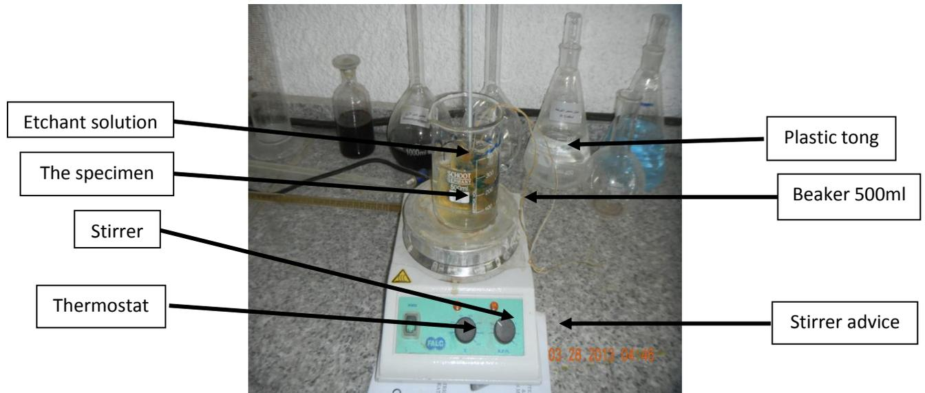
**Figure (2) Chemical machining system.**
