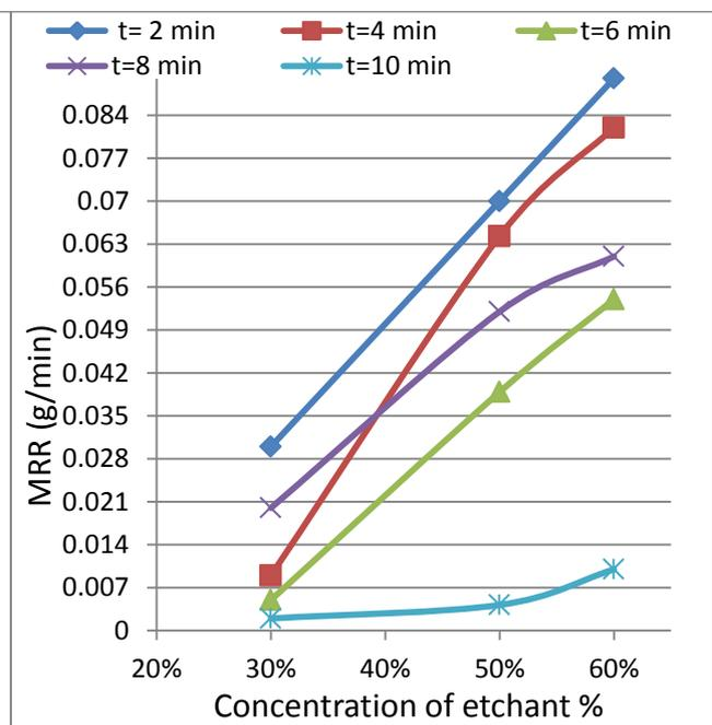
Figure (6) Effect of etchant concentration on MRR
