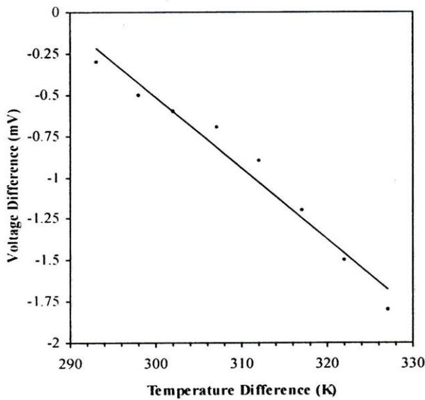
Fig.(3) : Thermovoltage as a function of temperature.
