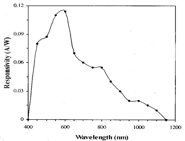
Fig.(7) : Spectral responsivity for SnO<sub>2</sub>/InP.
