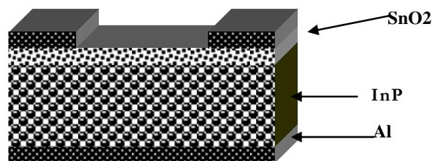
**Fig.(1) : Cross-sectional view of heterojunction.**
