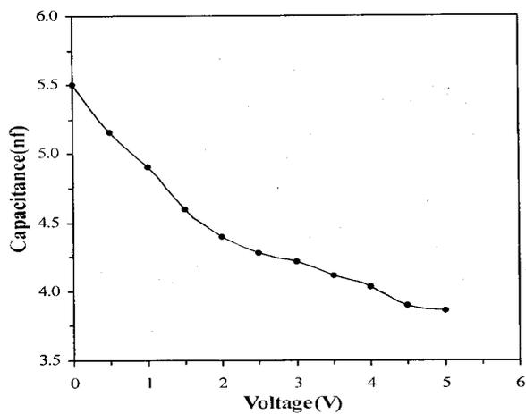
Fig.(4) : Capacitance vs reverse voltage curve.
