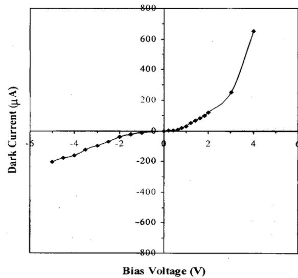
Fig.(6) : The I-V characteristic of SnO<sub>2</sub>/InP cell under dark condition.
