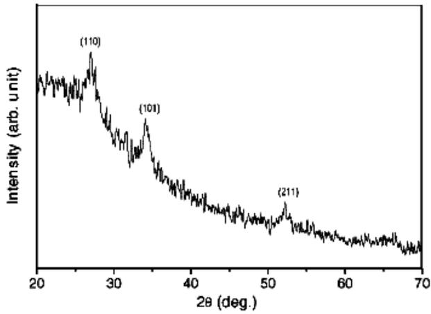
Fig.(2) : XRD patterns of the SnO<sub>2</sub> films on glass substrate.
