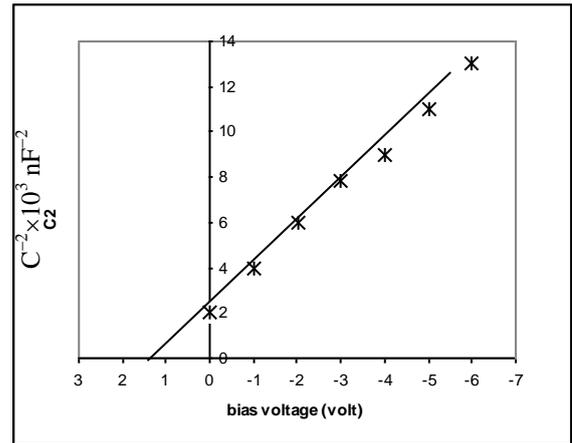
Fig.(5) :  $C^{-2}$  versus Bias voltage for characteristics SnO<sub>2</sub>/InP heterojunction.
