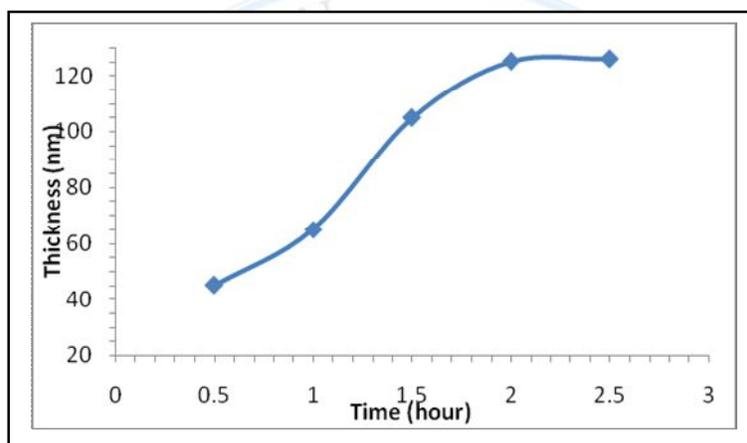
**Figure 1: shows variation of ZnS film thickness with different deposition time**
