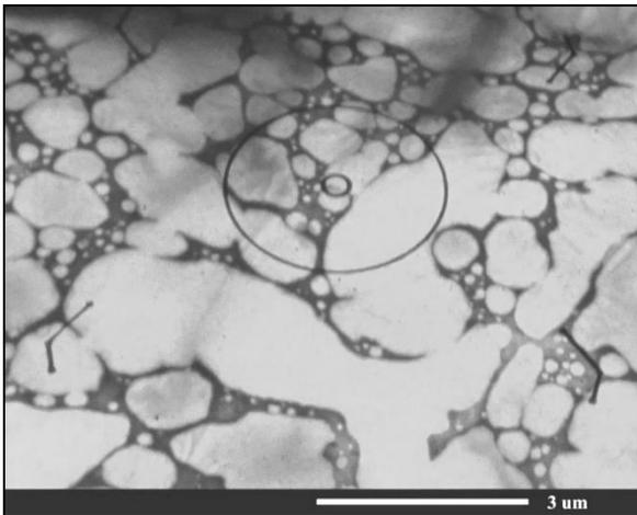
Figure 2: The TEM image of the non-inverted copper grids sample, the microbubbles could not be recognized. Instead, they appear as an irregular structures.
