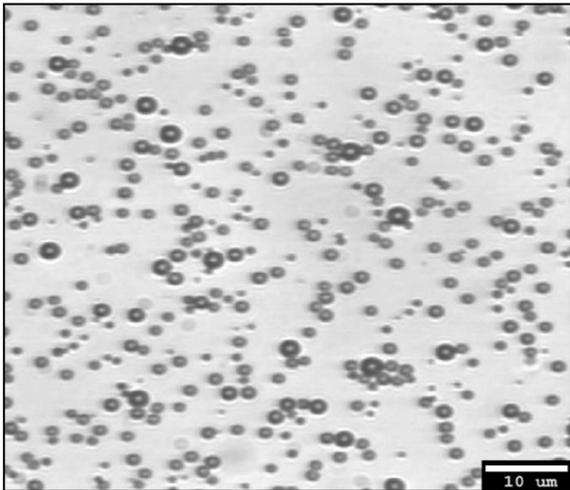
Figure 1: The image of the microbubbles obtained from optical microscopy
