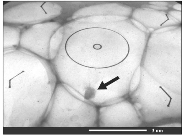
Figure 3: The TEM image of the microbubbles for the inverted copper grids sample. It's clearly showed the microbubbles that were resist the vacuum of TEM and accumulated on each other. Black arrow shows an area that could be residue of the staining with uranyl acetate
