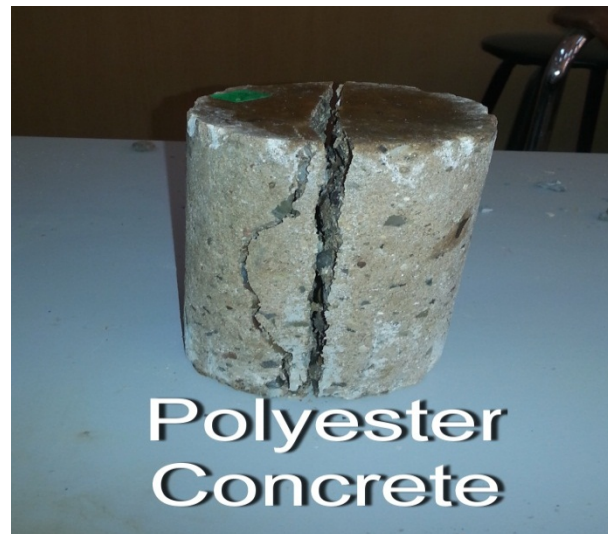
Figure(4) the polyester resin concrete specimens after splitting tensile test.
