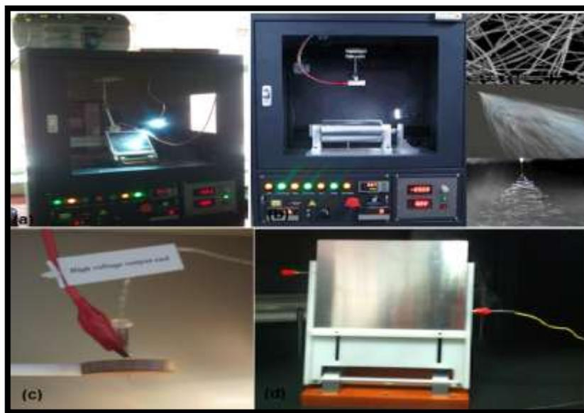
Figure(2): **a)**Nanobond Electrospinning system with rotation collector, **b)**with flat plate collector, **c)** needle connected to high voltage by upper electrode .,and **d)** flat aluminum plate collector connected to earthing lower electrode, with Taylor cone and spun image .
