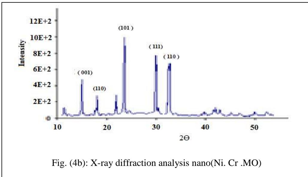
Fig. (4b): X-ray diffraction analysis nano(Ni. Cr .MO)
