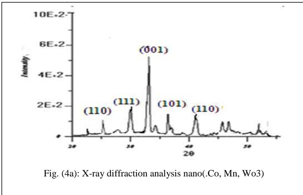
Fig. (4a): X-ray diffraction analysis nano(.Co, Mn, Wo3)
