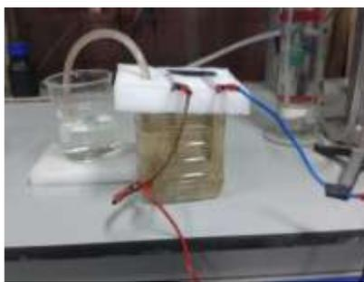
Fig. (5b) laboratory work shows hydrogen Production on nano electrode (Aluminum oxide)
