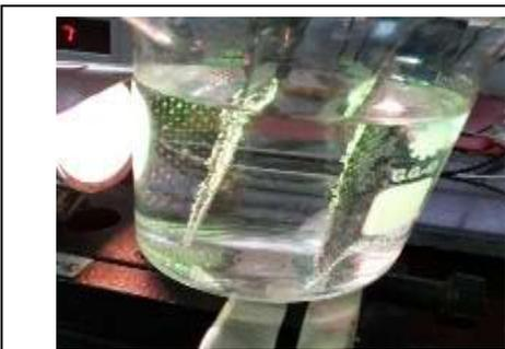
Fig. (5a) laboratory work shows hydrogen Production on nano electrode (glass )
