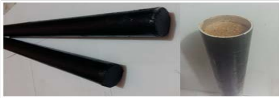
Figure (3) Sealing cylindrical capsules and packing of combined SHS m and LHS m
