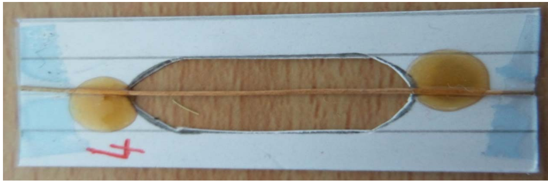
Figure (4): Stiff card sheets frame corn fiber sample for Single-fiber tensile test.
