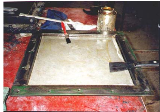
Plate (4): Furnishing and oiling light gauge base of the form.
