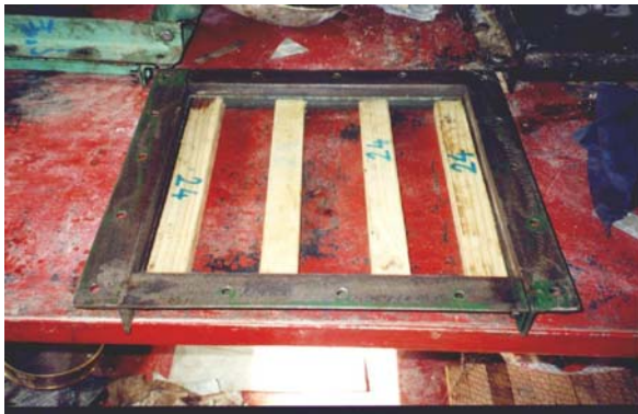
Plate (3): Specimen thickness control.
