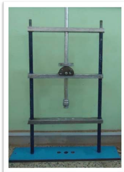
Plate (2): Piles hammer device.
