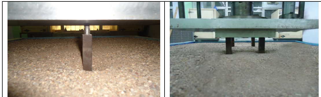
Figure (4): Installation of model piles.
