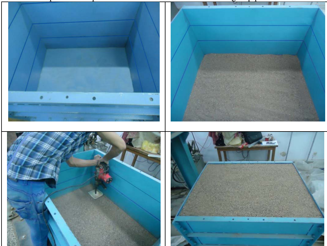
Figure (3): represents the sand deposit preparation.
