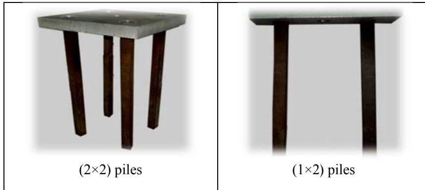
Plate (3): Piled cap configuration
