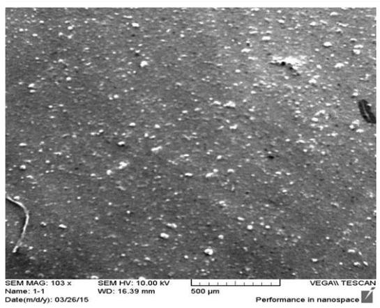
**Fig.(2): SEM, Analysis Ag nanoparticles synthesis by of the *N. oleander*.**
