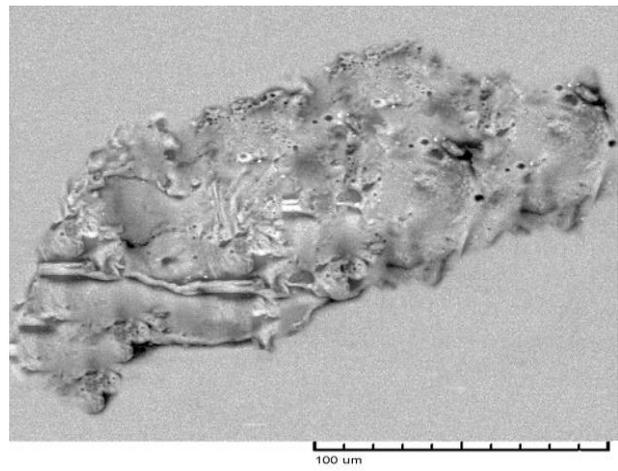
**Fig.(6):** SEM image of Al on Si substrate at 10 J/cm<sup>2</sup>.
