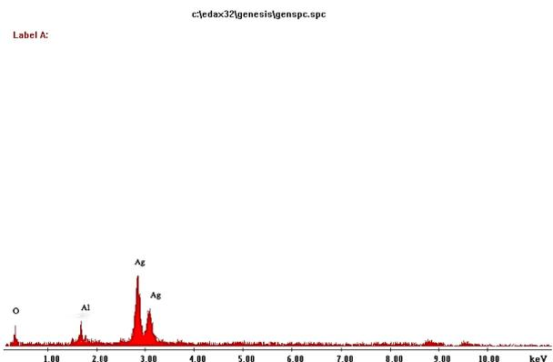
**Fig.(5):** EDAX spectrum of the deposition of Al thin film on Ag substrate.
