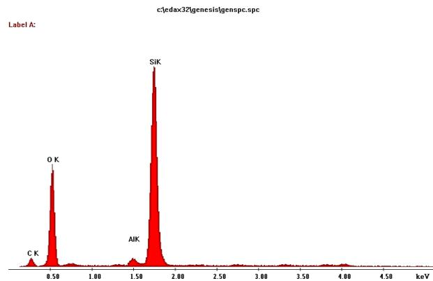
**Fig.(7):** EDAX spectrum of the deposition of Al thin film on Si substrate.
