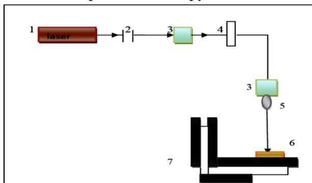
**Fig.(1): Scheme of Laser Induced Forward Transfer setup**
