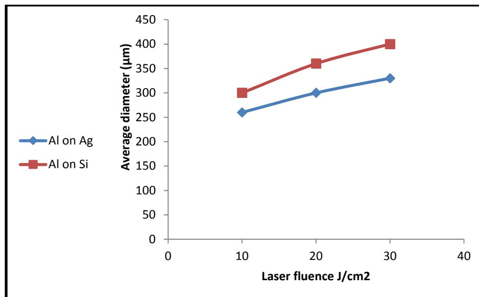
*Fig.(8): Diameter of the deposited dots plotted as a function of the laser fluence for Al on Ag and Si substrates.*
