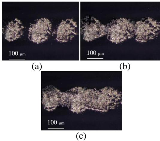
**Fig.(3):** Optical Microscopy images of Al thin film on Si substrate deposition at different laser fluencies: (a) at 10 J/cm<sup>2</sup>, (b) 20 J/cm<sup>2</sup> and (c) 30 J/cm<sup>2</sup>.
