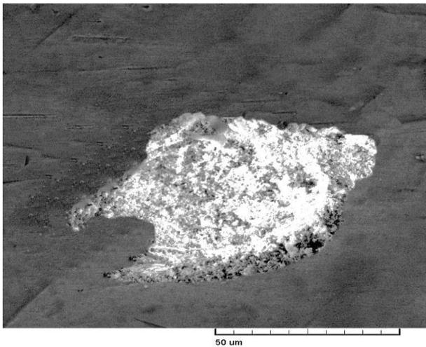
**Fig.(4):** SEM image of Al thin film on Ag substrate at 10 J/cm<sup>2</sup>.
