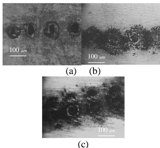
**Fig.(2): Optical Microscopy images of Al thin film on Ag substrate deposition at different laser fluencies: (a) at  $10 \text{ J/cm}^2$ , (b)  $20 \text{ J/cm}^2$  and (c)  $30 \text{ J/cm}^2$ .**
