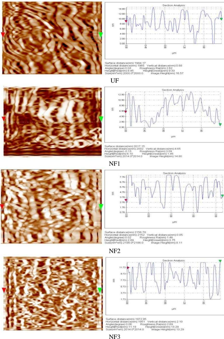
**Fig. 2. Two dimensions AFM images of the UF and NF membranes.**
