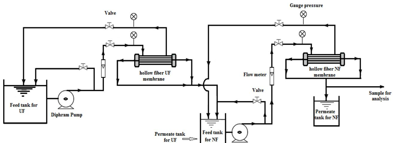
Fig. 1. Schematic diagram of the raw produced water treatment system.
