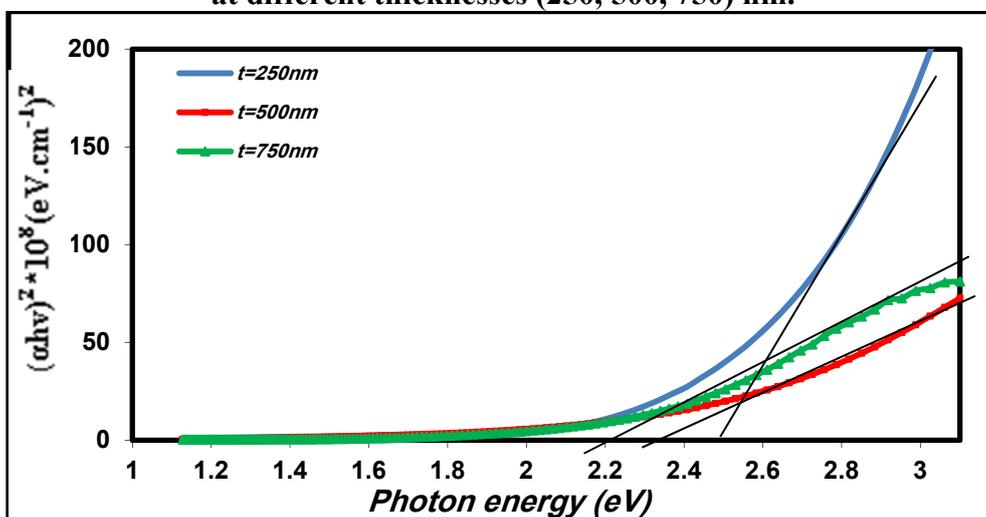
Figure (6) Variation of  $(\alpha h\nu)^2$  with photon energy for AgAlSe<sub>2</sub> thin films at different thicknesses (250, 500, 750) nm.
