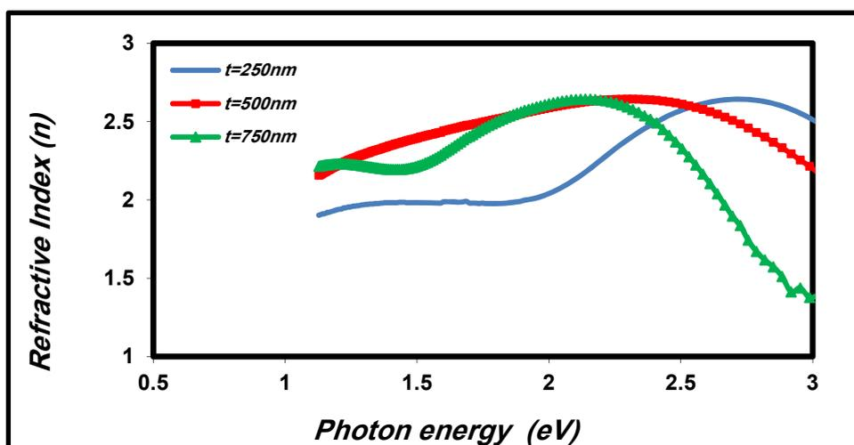
Figure (7) Variation of refractive index with photon energy for AgAlSe<sub>2</sub> thin films at different thicknesses (250, 500, 750) nm.
