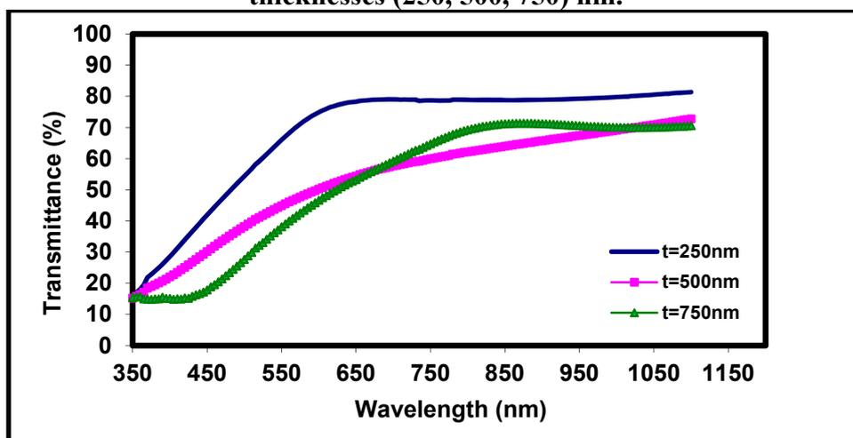
Figure (3) Transmittance spectra for  $AgAlSe_2$  thin films at different thicknesses (250, 500, 750) nm.
