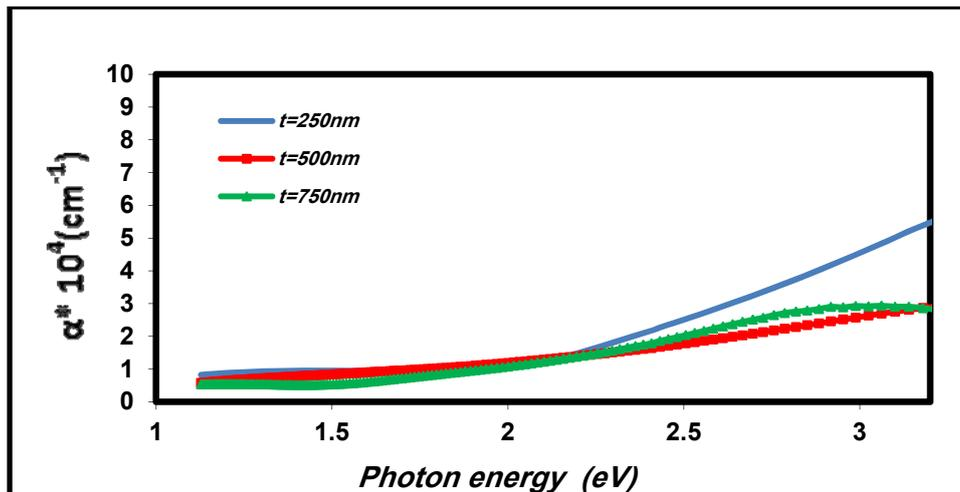
Figure (5) Variation of absorption coefficient with photon energy for AgAlSe<sub>2</sub> thin films at different thicknesses (250, 500, 750) nm.
