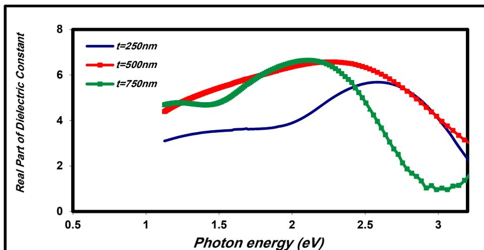
Figure (9) Variation of *real part of dielectric constant* with photon energy for  $\text{AgAlSe}_2$  thin films at different thicknesses (250, 500, 750)nm.
