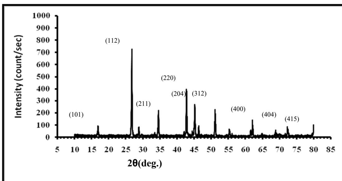
Figure (1) X-ray diffraction pattern of AgAlSe<sub>2</sub> alloy.
