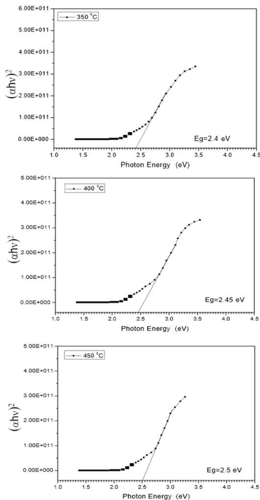
Fig. 5 (continue).  $(\alpha h\nu)^2$  versus wavelength of different substrate temperature.
