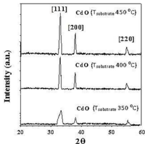
Fig. 1. XRD of CdO of different substrate temperature.
