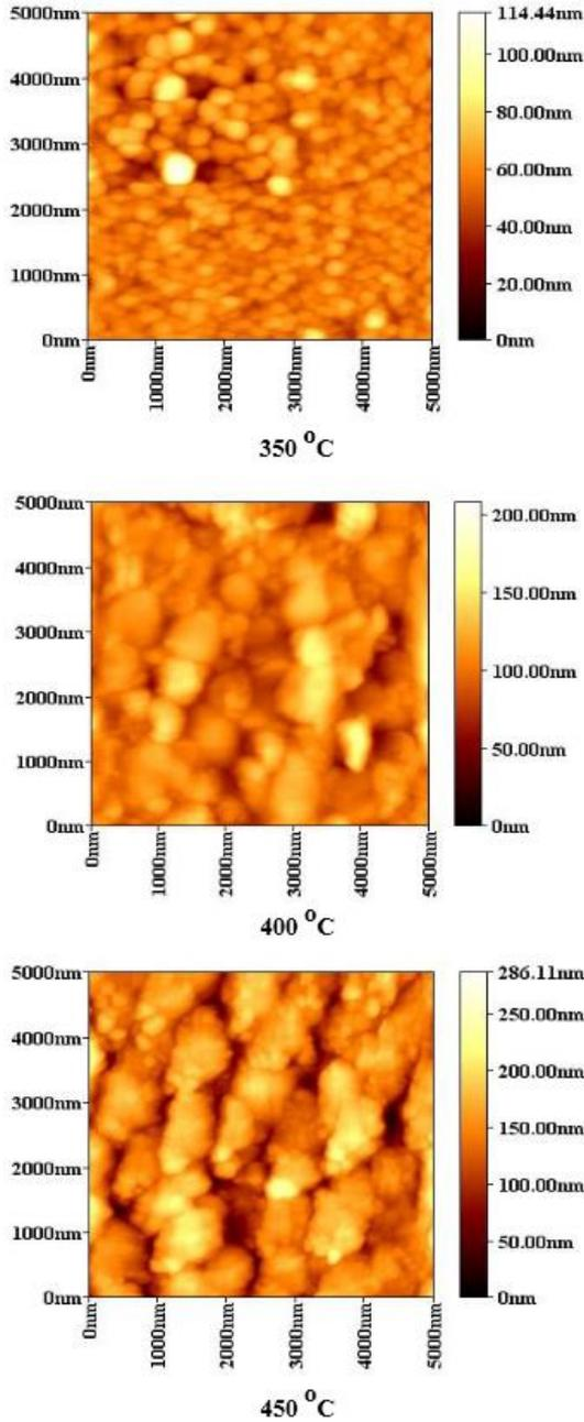
Fig. 2. AFM images for CdO thin films of different substrate temperature.
