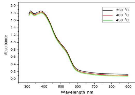
Fig. 4. Absorbance versus wavelength of different substrate temperature.
