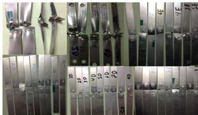
Figure (5) the tested shear force specimen
